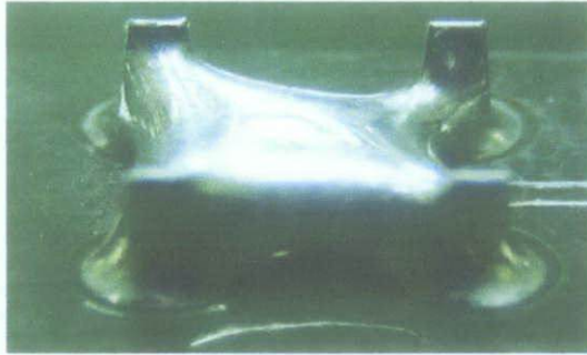
Figure 2: Solder bridging defect
