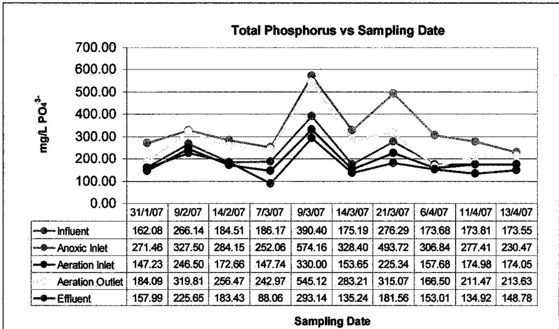
**Figure 11: Graph of Total Phosphorus versus Sampling Date after Rectification**
