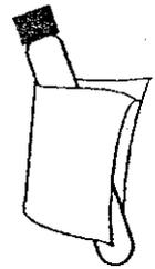
**16.** After the timer beeps, wipe the outside of the vial with a damp cloth followed by a dry one, to remove fingerprints or other marks.
