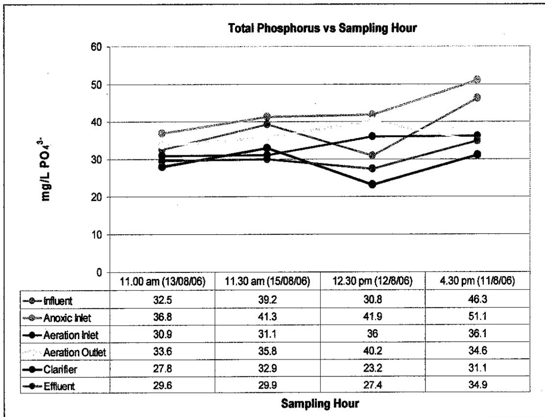
**Figure 9: Graph of Total Phosphorus versus Sampling Hour before Rectification**
