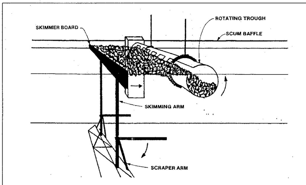
**Figure 8: Typical Rotating Skimmer Device**
