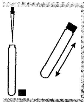
Use a TenSette Pipet to add 2 mL of 1.54 N Sodium Hydroxide Standard Solution to the vial. Cap and mix.
