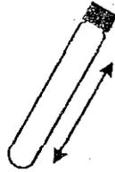
**14.** Cap tightly and shake to mix for 10–15 seconds. The powder will not dissolve completely.
