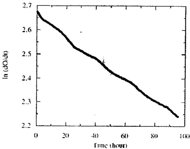
**Figure 13.** Endogenous decay rate,  $k_d$ , determination with well washed activated sludge.
