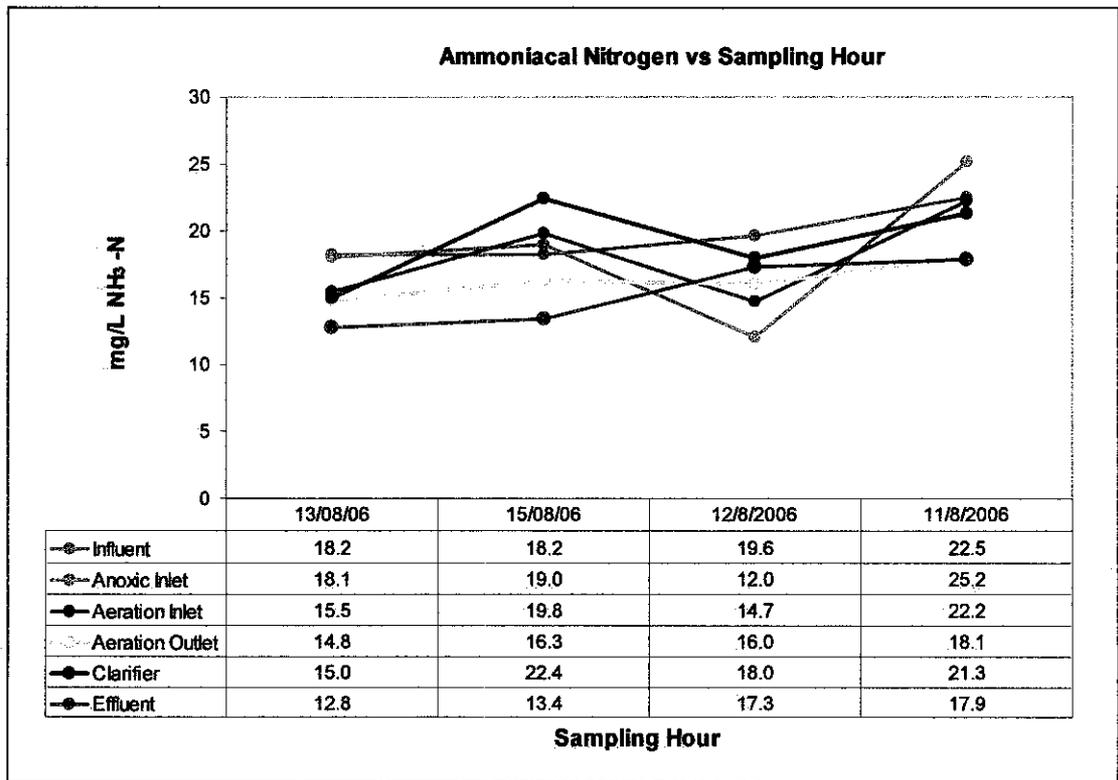
**Figure 13: Graph of Ammoniacal Nitrogen versus Sampling Hour before Rectification**
