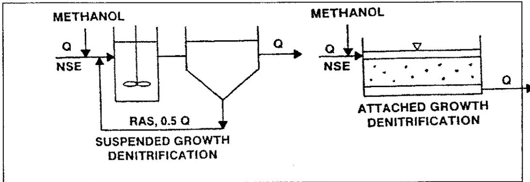
Figure 3: Separate Stage Nitrogen Removal System (Sedlak, 1991)
