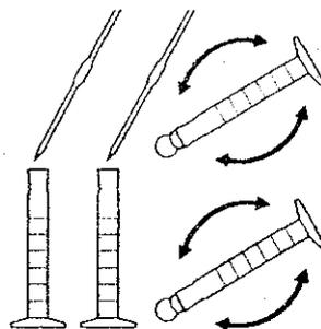
7. Pipet 1.0 mL of Nessler Reagent into each cylinder. Stopper and invert several times to mix.
