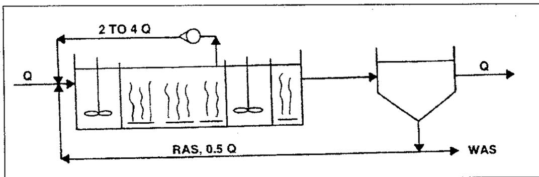
Figure 4: Single Sludge Nitrogen Removal System (Sedlak, 1991)
