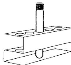
8. When the timer beeps, carefully remove the hot vial from the reactor. Place it in a test tube rack and cool to room temperature.
