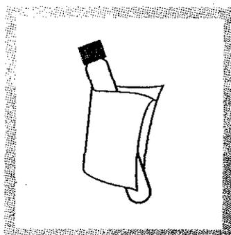
10. Wipe the outside of the vial with a damp cloth followed by a dry one, to remove fingerprints or other marks.
