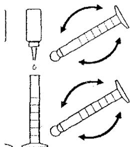
5. Add three drops of Mineral Stabilizer to each cylinder. Stopper and invert several times to mix.
