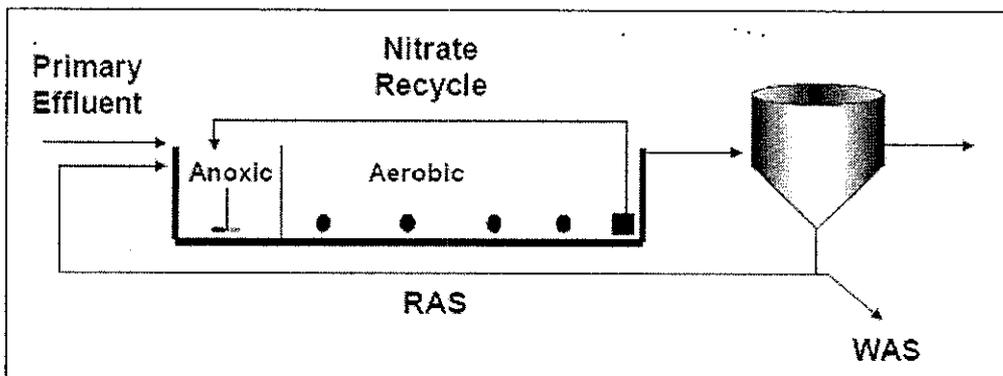
**Figure 6: Layout of UTP's Anoxic Zone**
