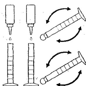
6. Add three drops of Polyvinyl Alcohol Dispersing Agent to each cylinder. Stopper and invert several times to mix.
