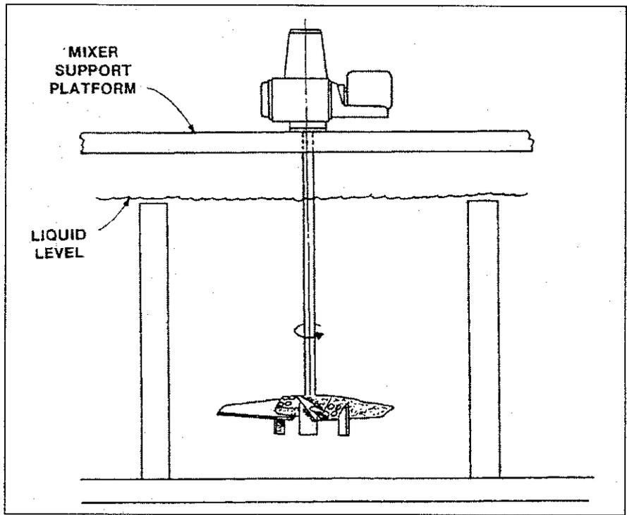
Figure 7: Typical Submerged Turbine Mixer
