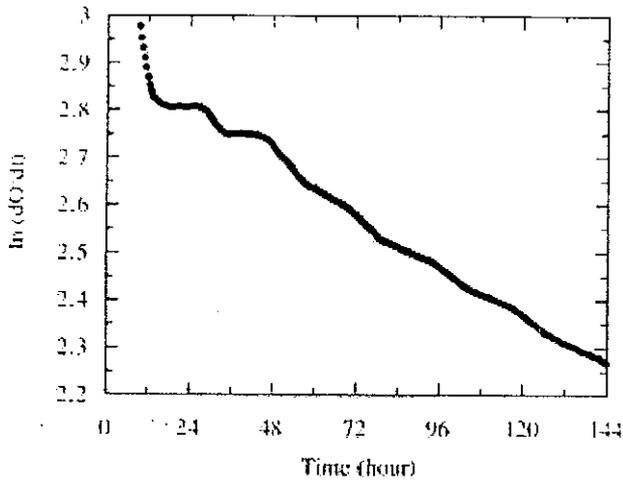
**Figure 12.** Endogenous decay rate,  $k_d$ , determination without well washed activated sludge.
