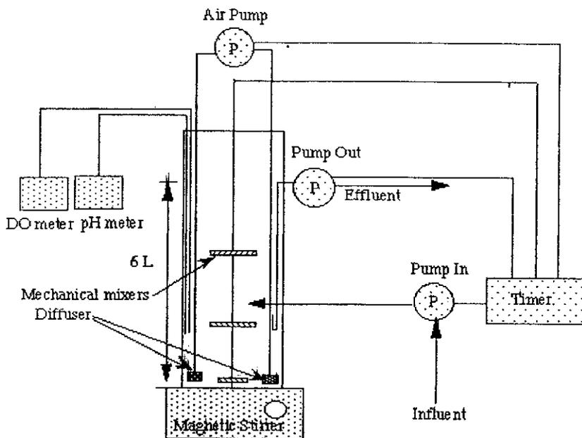
Figure 16. A typical SBR configuration.
