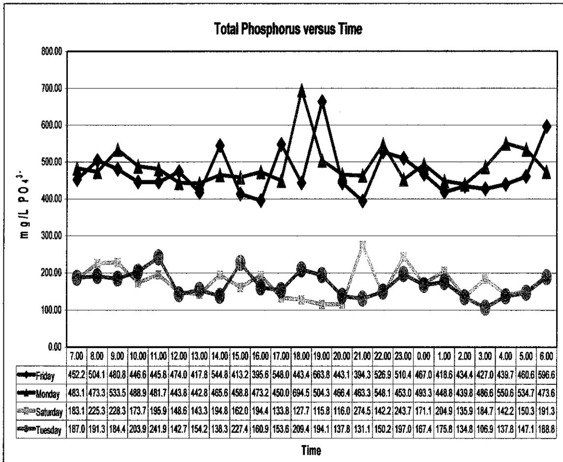
**Figure 18: Graph of Total Phosphorus Nitrogen Concentration in Influent of Oxidation Pond versus Time during Fasting Month**
