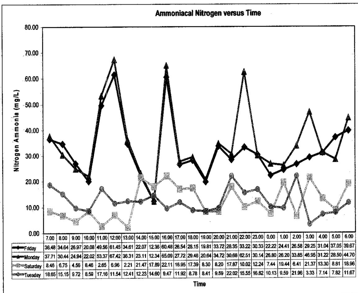
**Figure 19: Graph of Ammoniacal Nitrogen Concentration in Influent of Oxidation Pond versus Time during Fasting Month**
