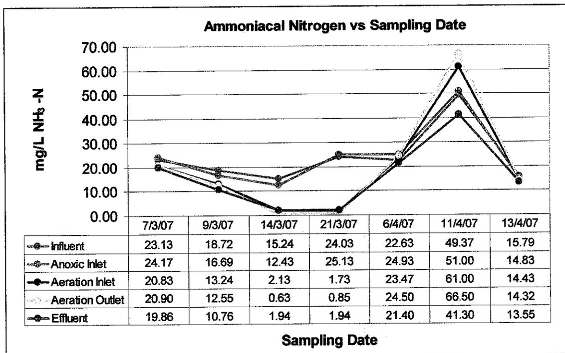
**Figure 15: Graph of Ammoniacal Nitrogen versus Sampling Date after Rectification**
