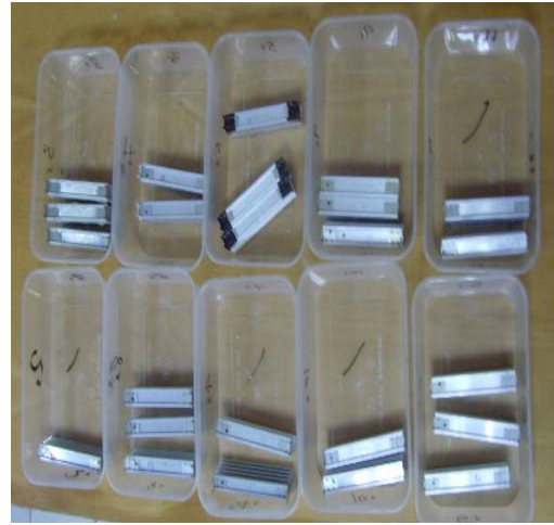
Figure A-10: Coated heat sink in simulated condition storage (Common room V5E)
