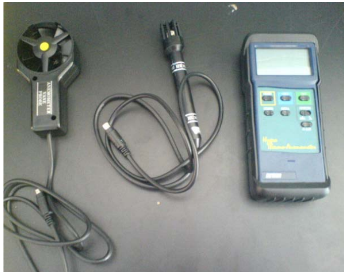
Figure 3-2: Data weathering instruments - Anemometer and Relative Humidity meter
