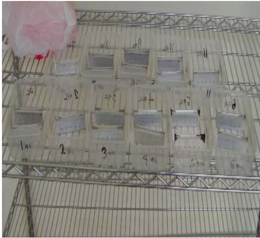
Figure A-9: Coated heat sink in accelerated condition storage (Block 15-00-02)
