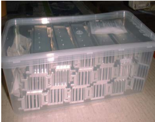
Figure A-26: Current packaging to prevent corrosion
