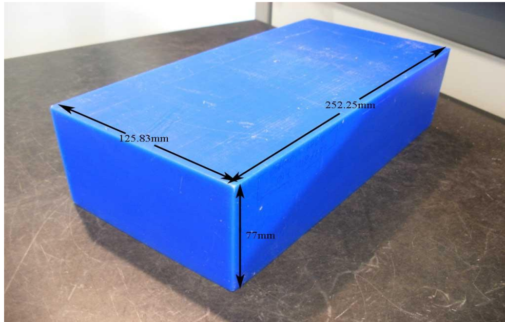
Figure 4-35: Wax piece is used as the raw material for machining
