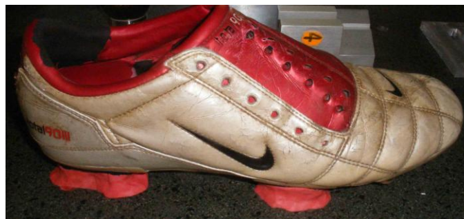
Figure 4-13: Mounted shoe using plasticine
