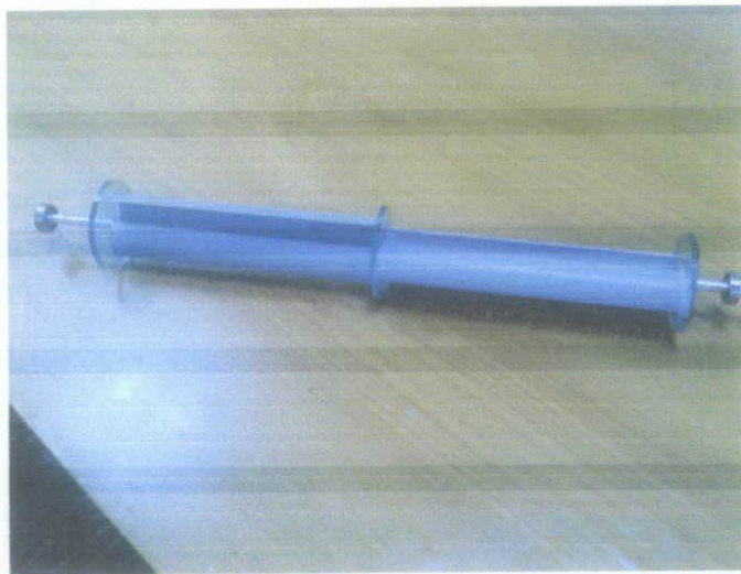
FIGURE 2.7: Savonius rotor prototype
