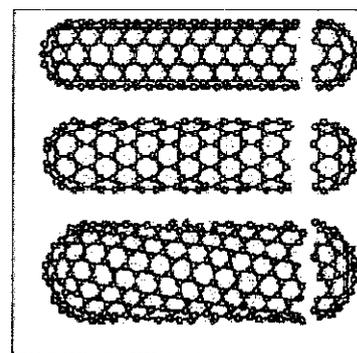
Figure 6-SWCNT Aromatic Structure
