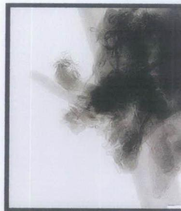
Figure 23- Pristine CNT Sample before Treatment
