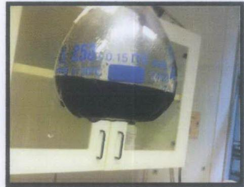
Figure 2 - Image captured at UTP lab of Dispersed MWCNTs after Step 3 ( Refer to Methodology)
