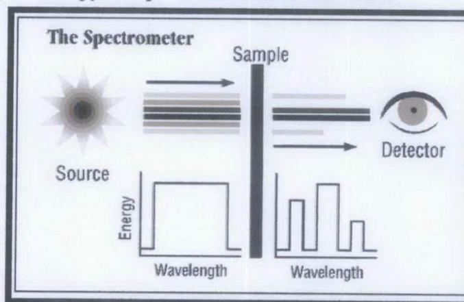
Figure 25- FT-IR spectroscopy Schematic Diagram
