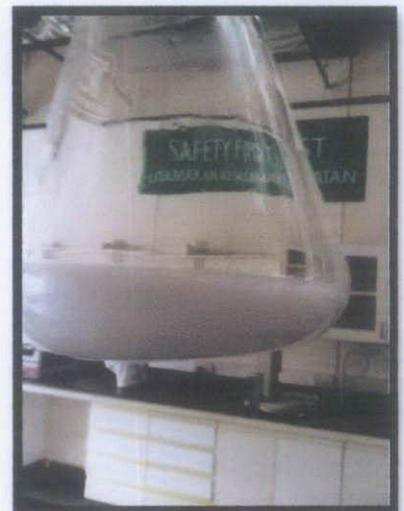
Figure 18- Prepared Sodium Zincate with excess Zinc Oxide Powder.
