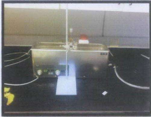
Figure 16 - UltraSonicator Bath Setup
