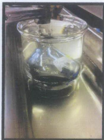
Figure 22- Mixture being Sonicated
