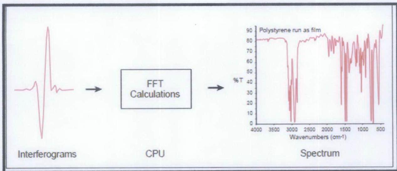
Figure 26-FT-IP spectroscopy Process
