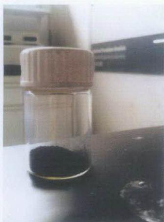
**Figure 12- 150mg of pristine MWCNT**
