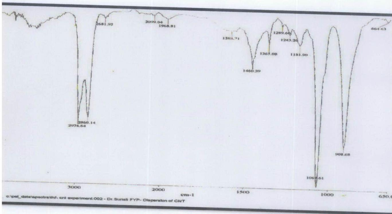
Figure 27-FT-IR of THF suspension
