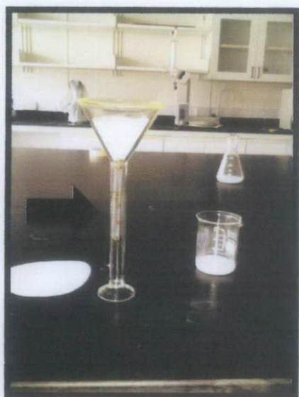
Figure 19- Filtering Unreacted Zinc Oxide
