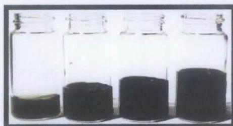
Figure 8- CNT in a THF suspension
