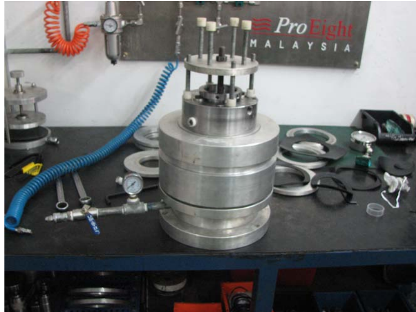
Figure 22: Pressure Test Equipment at ProEight Offshore Engineering Sdn. Bhd
