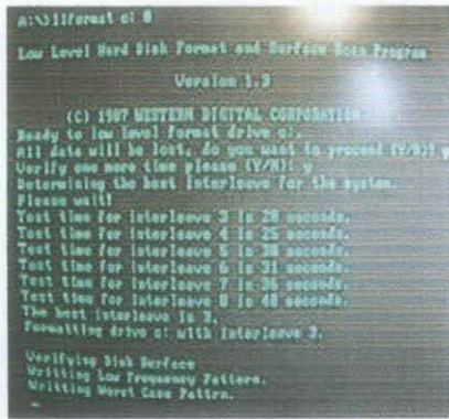
Figure 2: Low-level format utility performing interleave speed tests on a 10-megabyte IBM PC XT hard drive [31]
