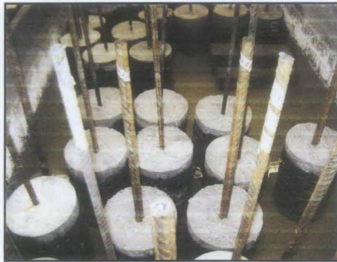
Figure 14 : Samples in the curing tank
