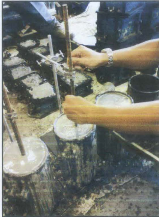
Figure 10 : Placing the steel bar inside the concrete
