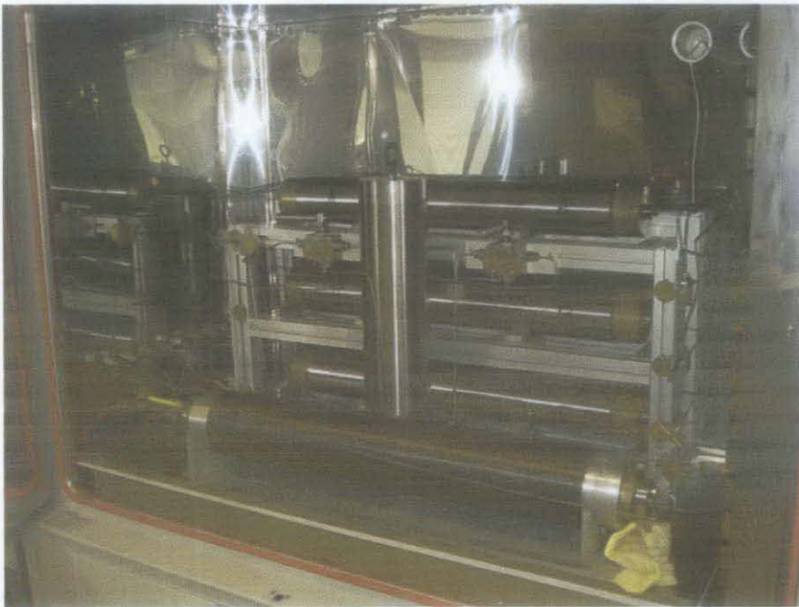
Figure 5: Relative Permeability Machine (Inside View)
