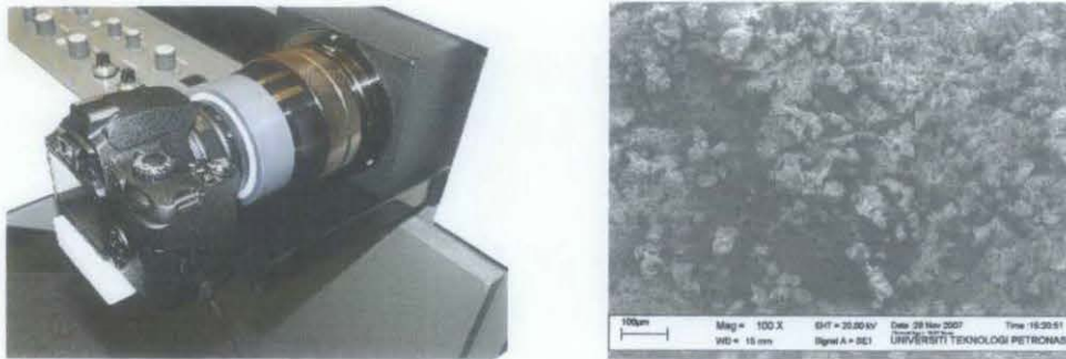
Figure 2.8: SEM testing machine and possible outcome of results
