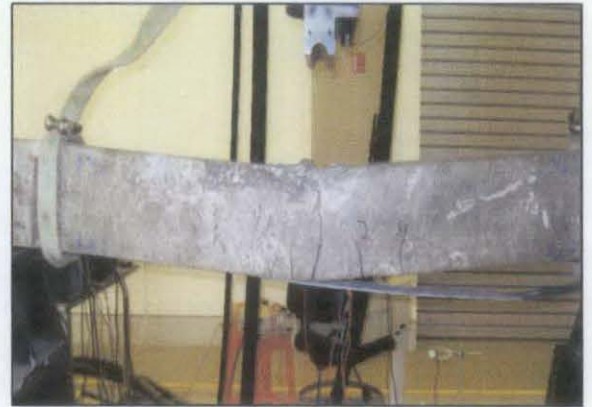
Figure 15 : Schematic Drawing and Picture of CB3 Crack Patterns
