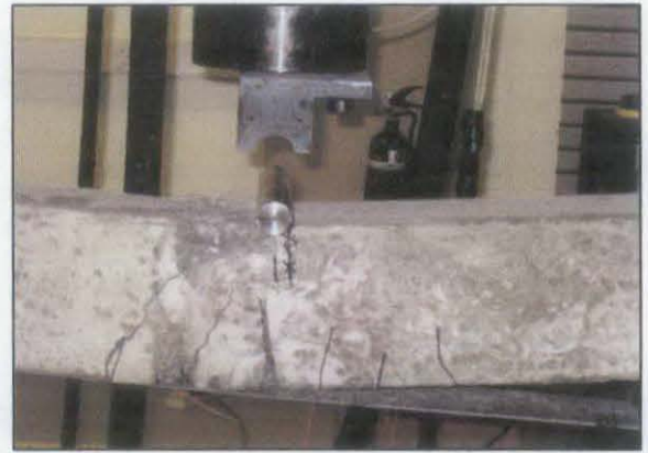
Figure 17 : Schematic Drawing and Picture of CB4 Crack Patterns
