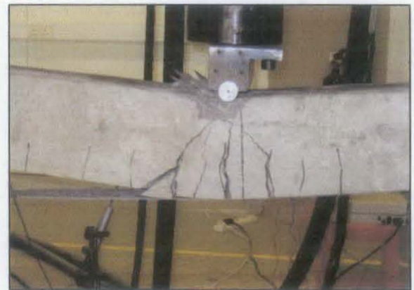
Figure 18 : Schematic Drawing and Picture of CF4 Crack Patterns
