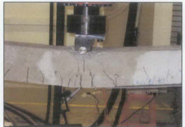
Figure 16 : Schematic Drawing and Picture of CF3 Crack Patterns
