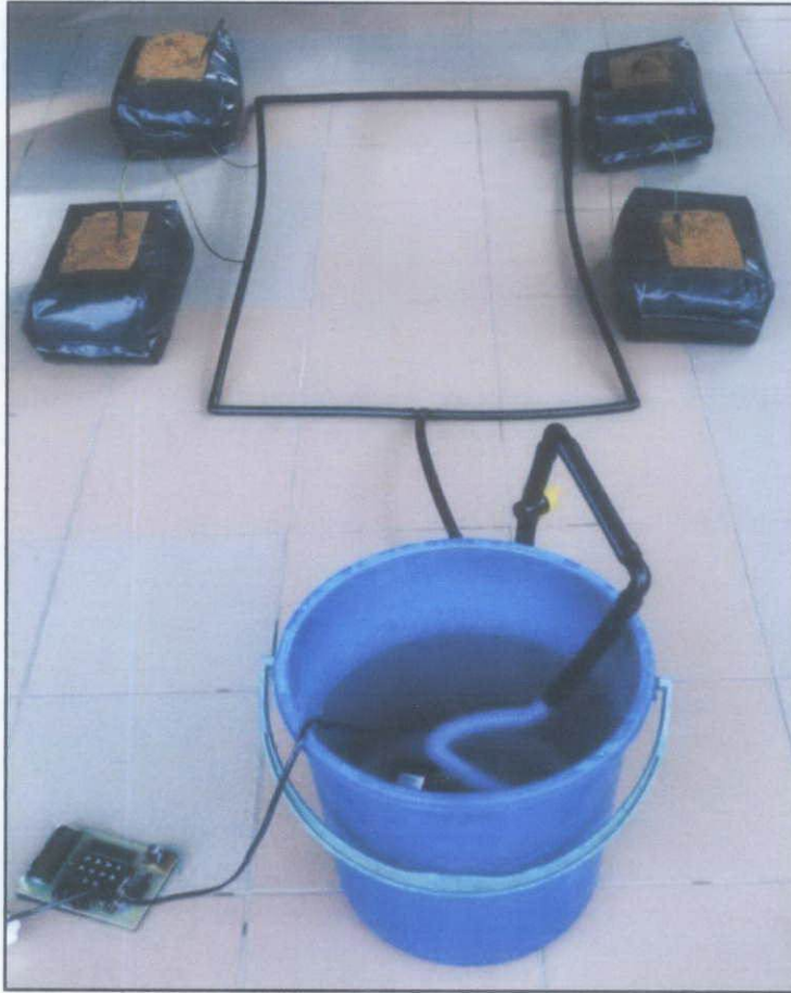
The Constructed Laboratory Model Fertigation System
