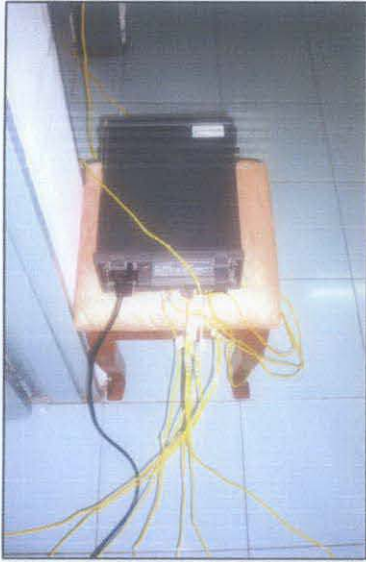
Figure 19: Data logger and anemometer set
