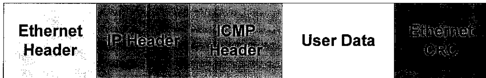
Figure 4: Example of an IP datagram carrying ICMP message for transmission over Ethernet
