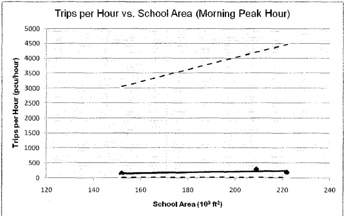
Figure 4.9 Graph trips per hour versus school area during morning peak hour (comparison with data given in Malaysian Trip Generation Manual)
