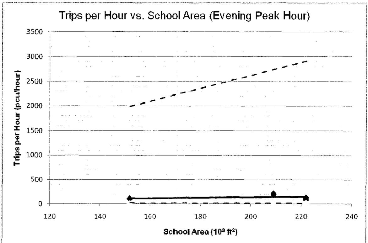
Figure 4.10 Graph trips per hour versus school area during evening peak hour (comparison with data given in Malaysian Trip Generation Manual)
