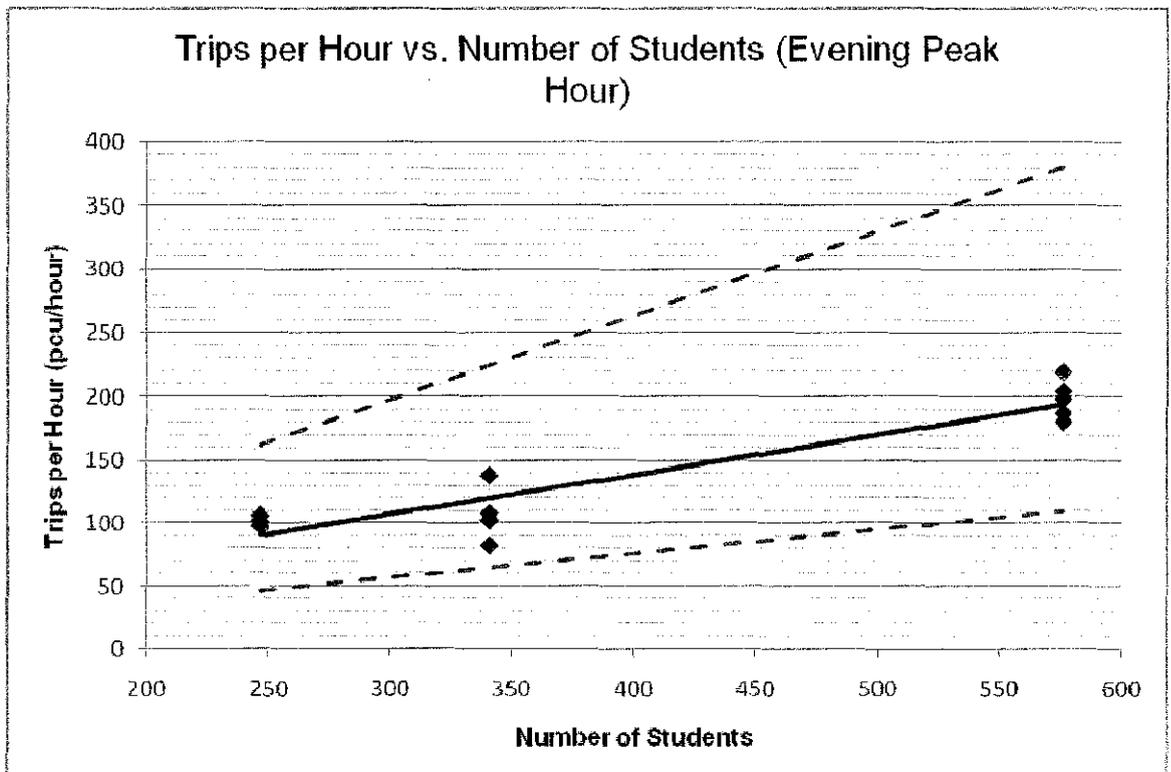
Figure 4.8 Graph trips per hour versus number of students during evening peak hour (comparison with data given in Malaysian Trip Generation Manual)
