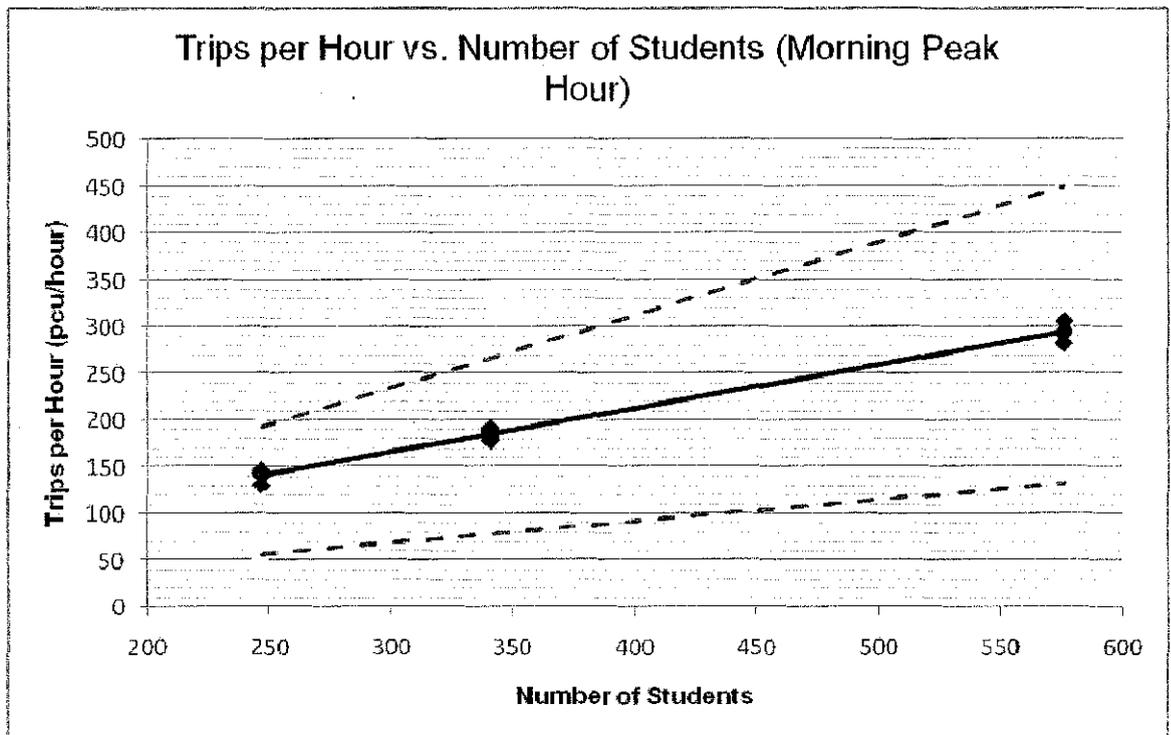
Figure 4.7 Graph trips per hour versus number of students during morning peak hour (comparison with data given in Malaysian Trip Generation Manual)
