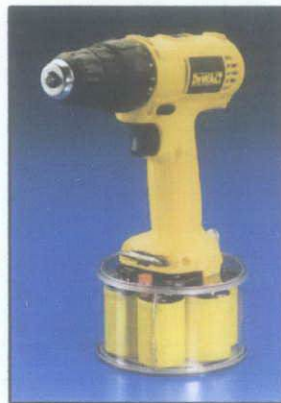
Figure 5: Cordless Drill Powered by Ultra-capacitor [16]
