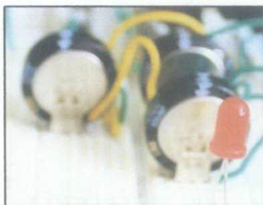
Figure 10: The 1F, 5.5V Ultra-capacitor
