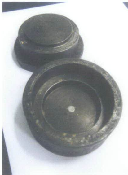
Figure B2: Compression molding mould
