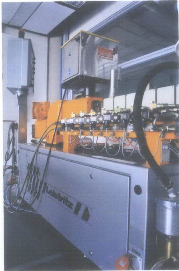
Figure B5: Twin screw extruder
