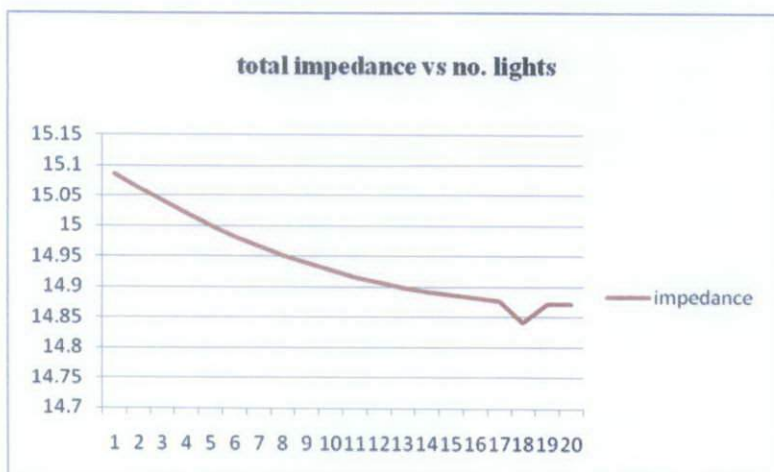
Figure 15 Graph for total impedance versus number of lights
