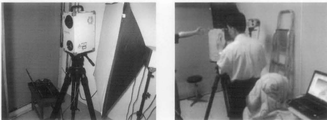
Figure 5-6: Set-up for capturing 3D images from patients
