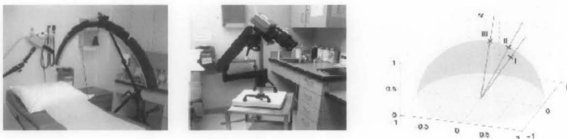
Figure 2-10: The light source and camera planted on arc and tripod moving in a hemisphere (reproduced from [Cula 2004])
