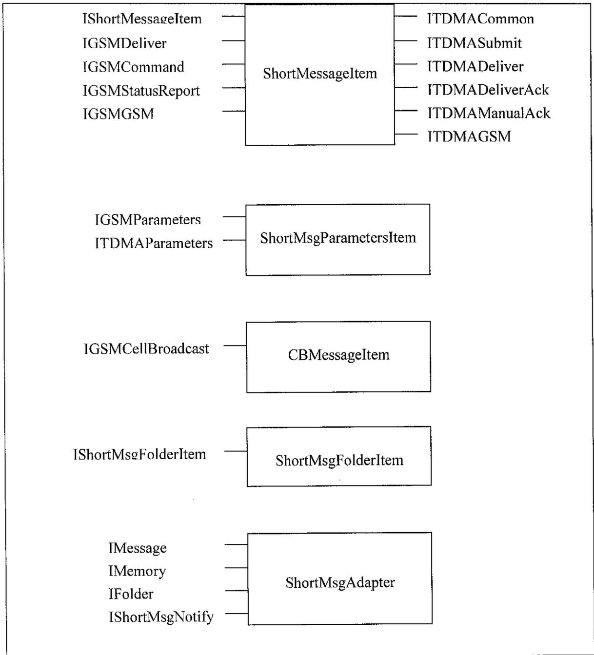
Figure 3-2: Components and interfaces of NclMsg.dll module
