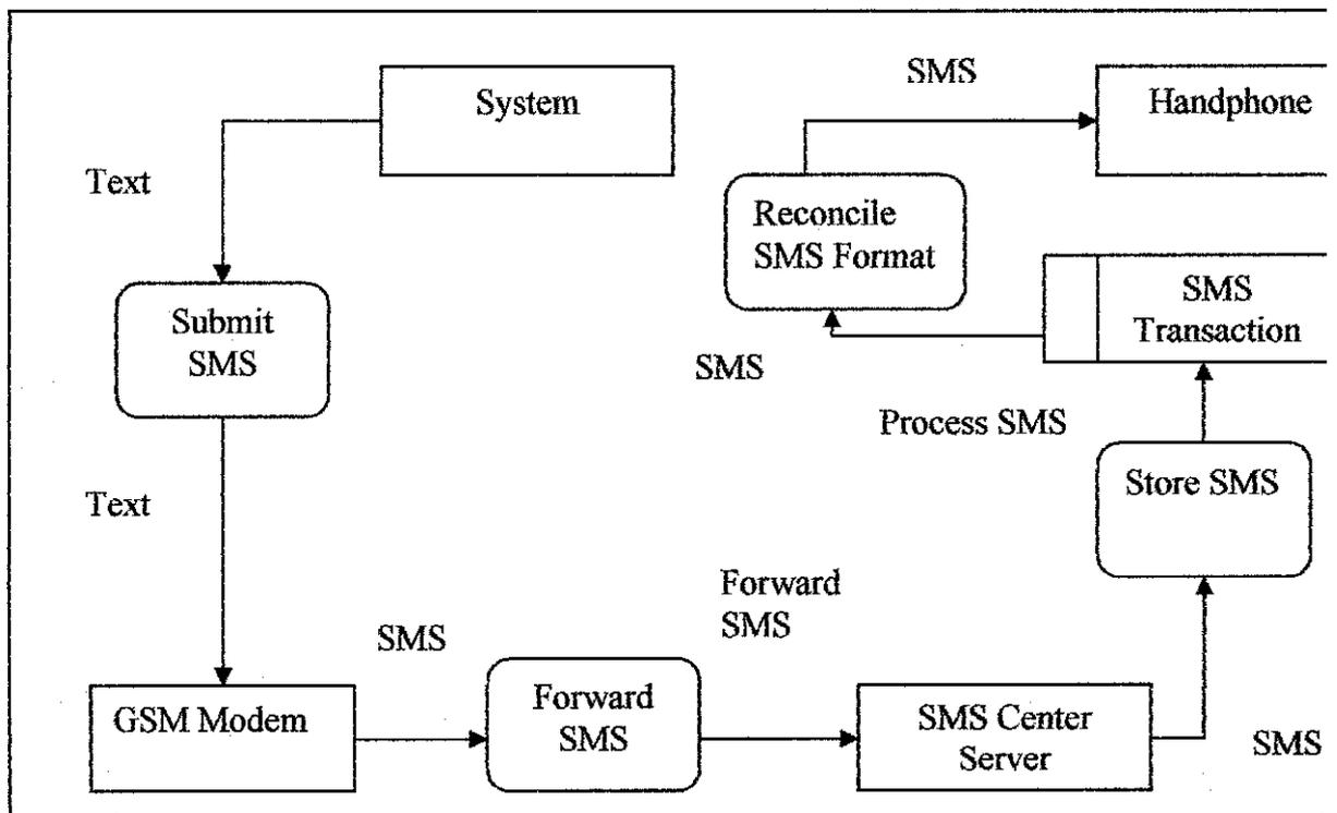
Figure 4-3: SMS Sending Data Flow Diagram
