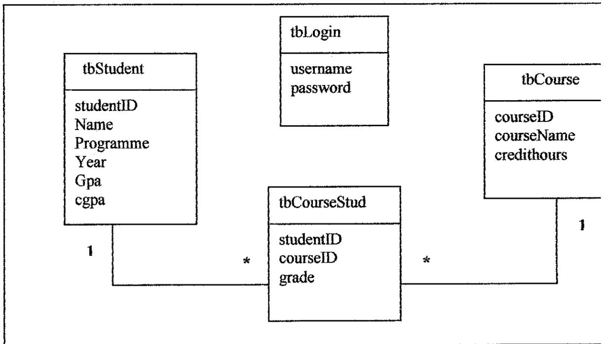
Figure 4-4: Class diagram for the student's examination result database
