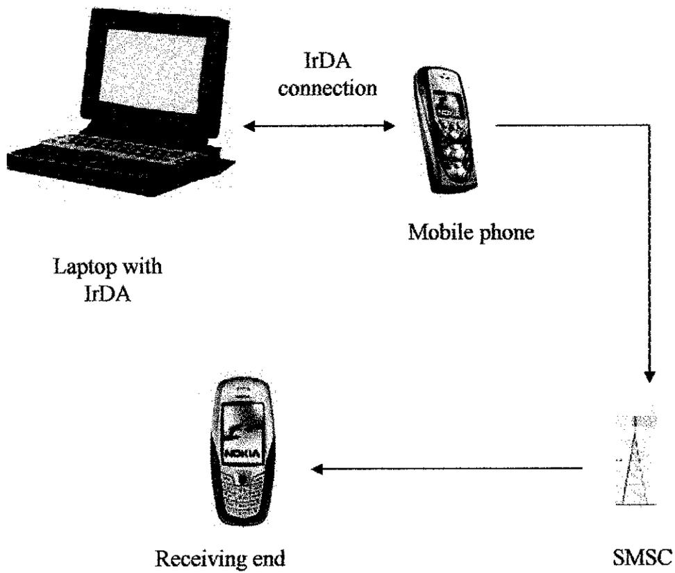
Figure 4-5: The flow of prototype
