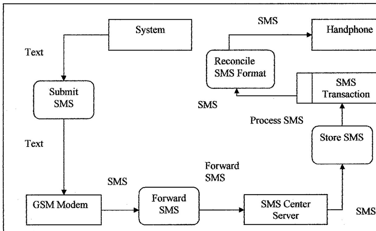
Figure 4-3: SMS Sending Data Flow Diagram
