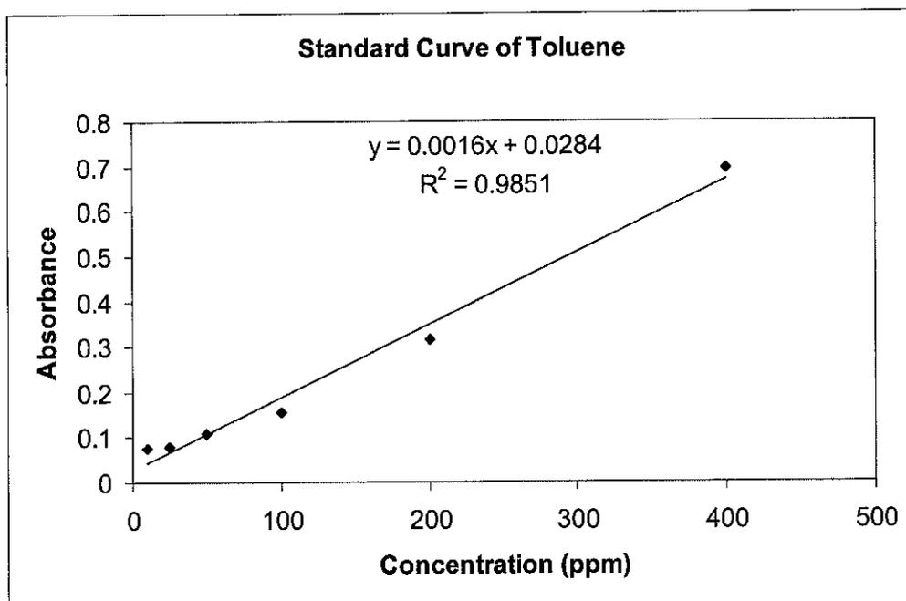
Figure 5.2: Calibration Curve of Toluene
