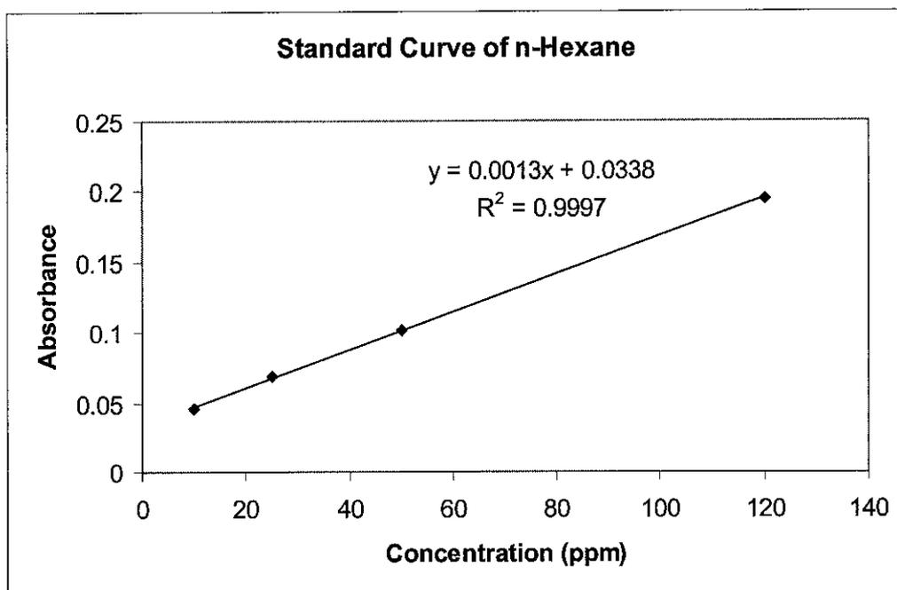
Figure 5.1: Calibration Curve of n-Hexane
