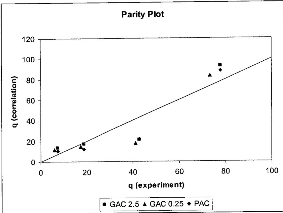
Figure 5.16: Parity Plot for Toluene Adsorption Isotherm at 35°C
