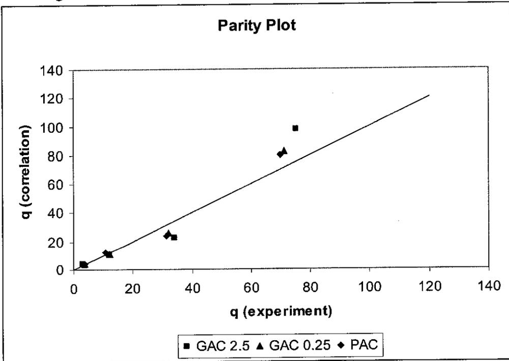
Figure 5.17: Parity Plot for Toluene Adsorption Isotherm at 55°C
