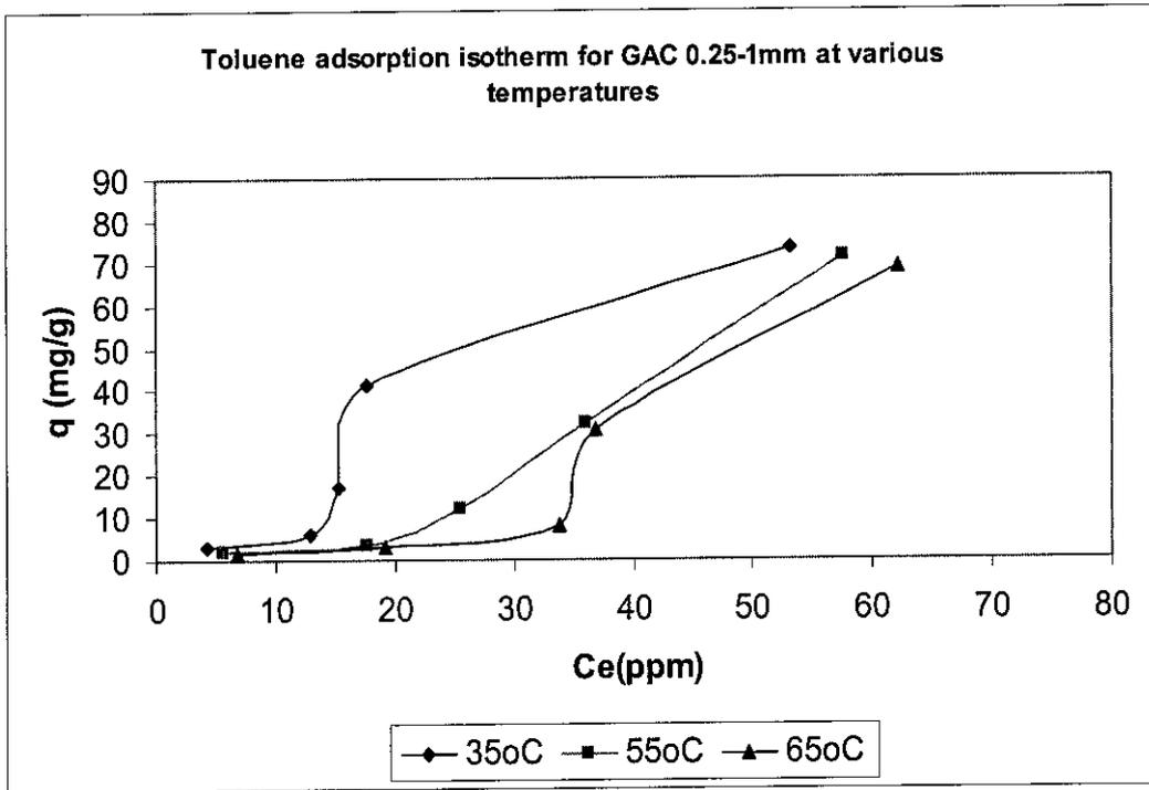
Figure 5.8: Toluene adsorption isotherm for GAC 0.25-1mm at various temperatures
