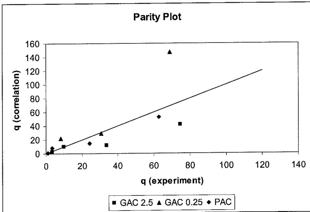
Figure 5.18: Parity Plot for Toluene Adsorption Isotherm at 65°C
