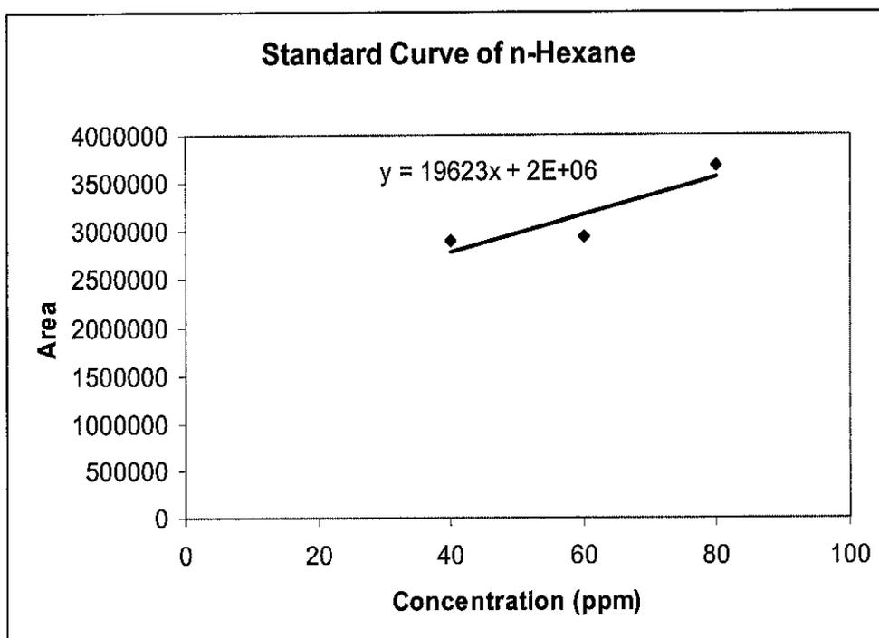
Figure 5.3: Calibration Curve of n-Hexane (for GCMS)
