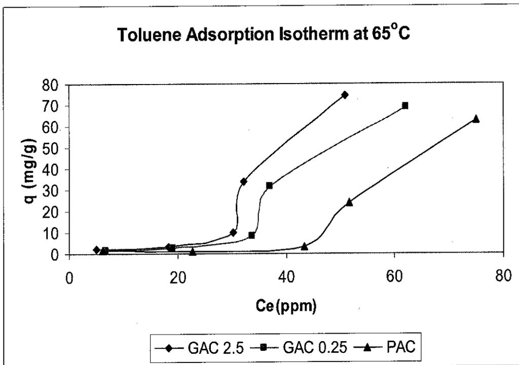
Figure 5.6: Toluene adsorption isotherm at 65°C
