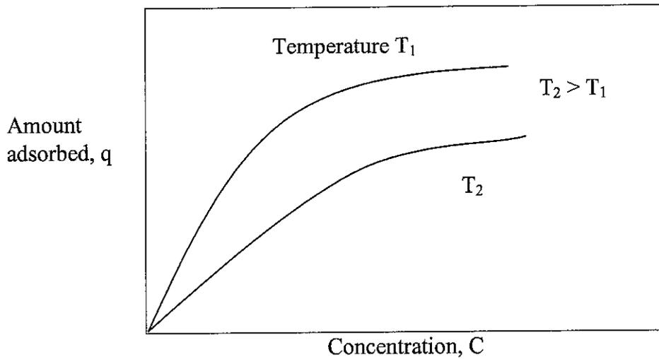
Figure 3.1: Adsorption Isotherm
