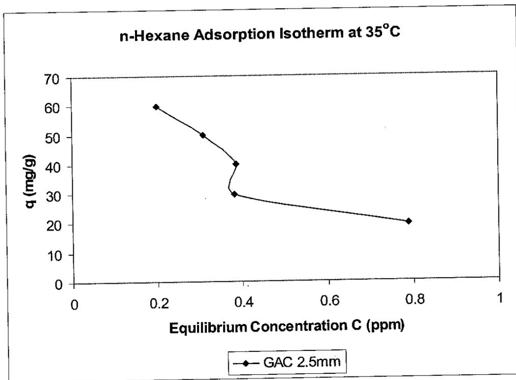
Figure 5.20: n-Hexane adsorption isotherm at 35°C (analyzing using GCMS)
