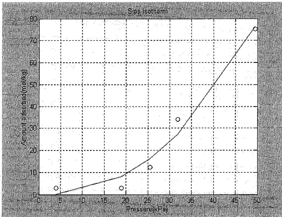
Figure 3: Sips isotherm at 65°C
