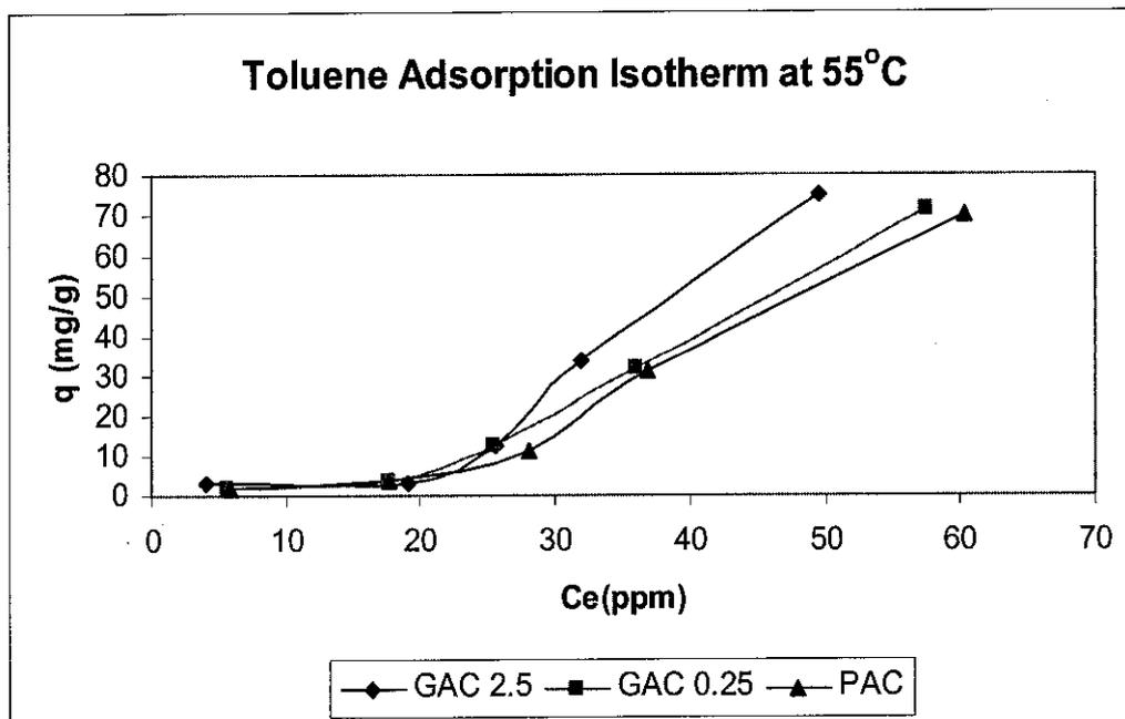
Figure 5.5: Toluene adsorption isotherm at 55°C
