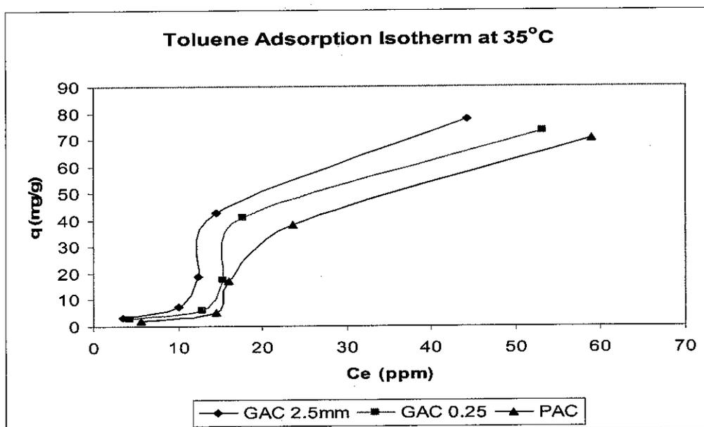
Figure 5.4: Toluene adsorption isotherm at 35°C
