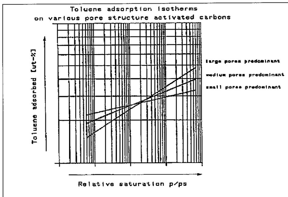
Figure 2.6: Idealized Toluene adsorption isotherm (Degel et al., 1990)
