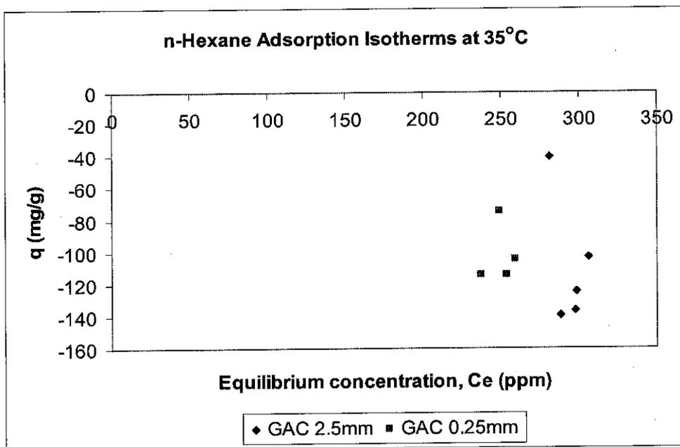
Figure 5.19: n-Hexane adsorption isotherm at 35°C (analyzing using UV-Vis Spectrophotometer)
