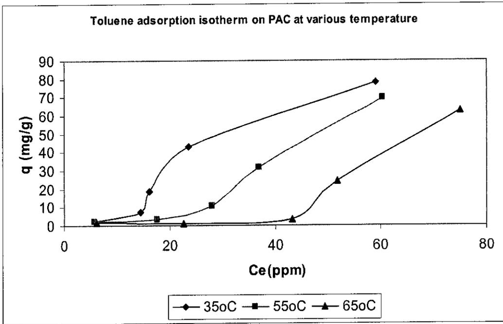
Figure 5.9: Toluene adsorption isotherm for PAC at various temperatures
