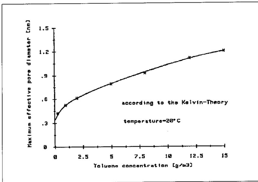
Figure 2.5: Relationship between pore size and toluene concentration (Degel et al., 1990)
