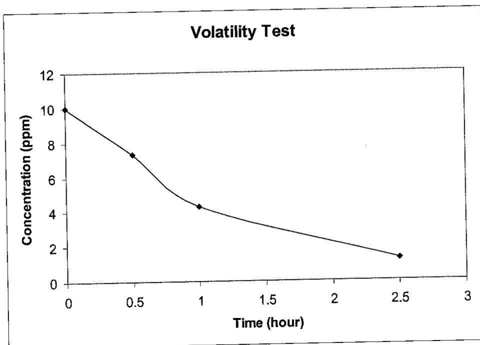
Figure 5.21: Volatility Test of n-Hexane
