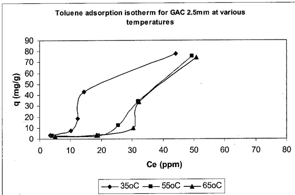
Figure 5.7: Toluene adsorption isotherm for GAC 2.5mm at various temperatures
