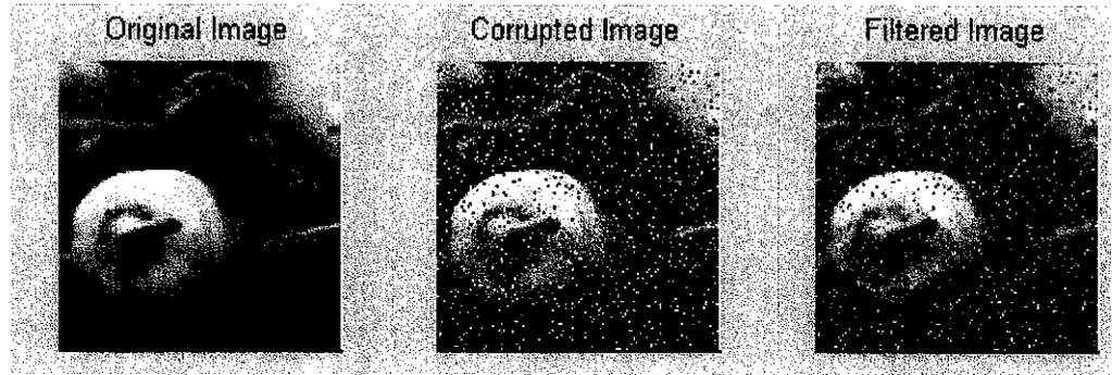
Figure 5 Effect of adaptive filter on salt and pepper noise
