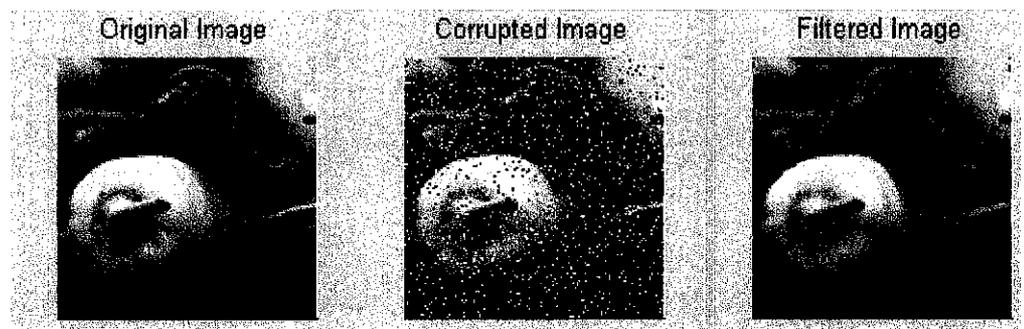
Figure 4 Effect of median filter on salt and pepper noise
