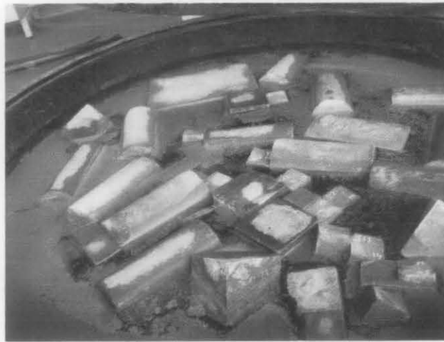
Figure 5: Mortar in water tank
