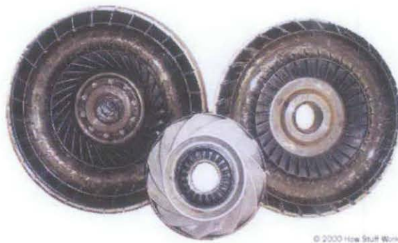
Figure 1.2: Torque converter components (from left to right); turbine, stator, pump.
