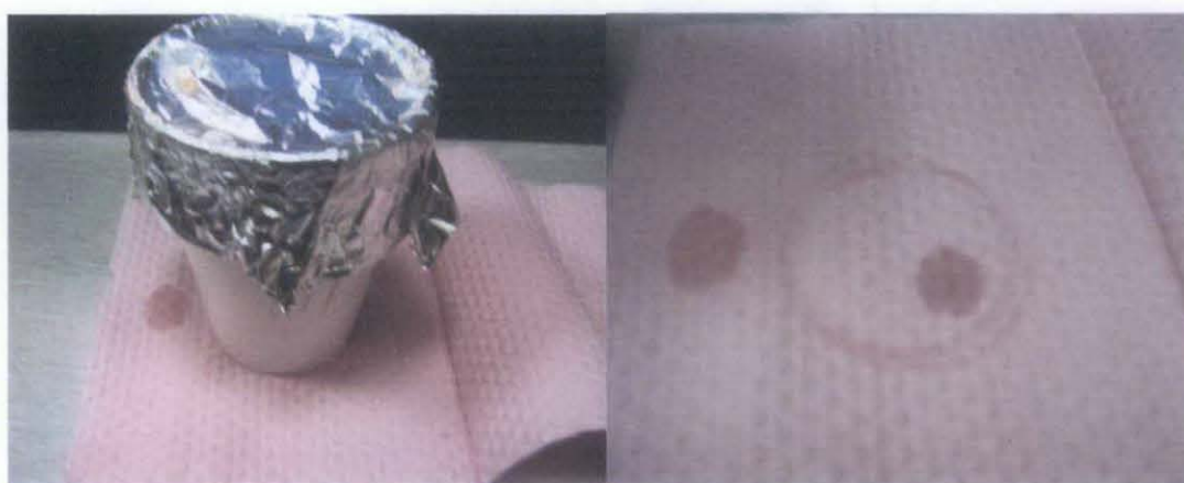
Figure 4.9: Oil marks on tissue paper, indicating cooking oil penetrating through the PS cup.
