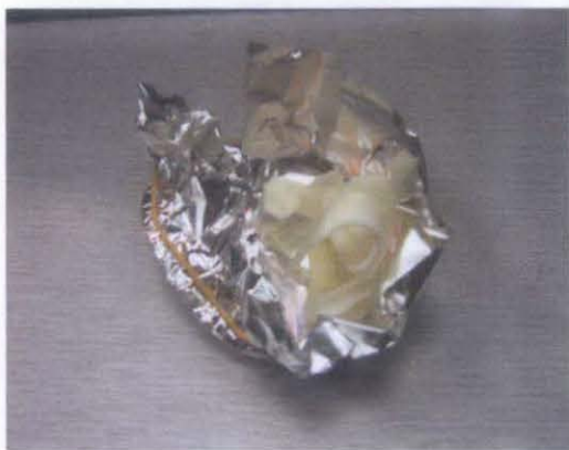
Figure 4.11: Ruptured PS cup at 125°C.
