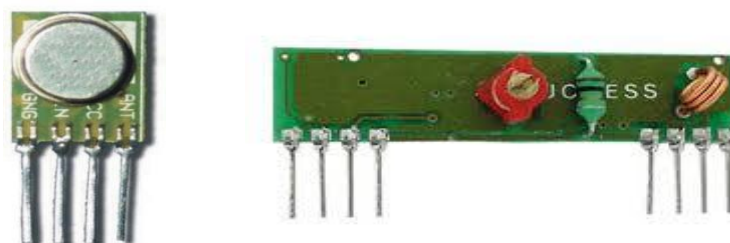
Figure 10: The transmitter and receiver for RF module.
