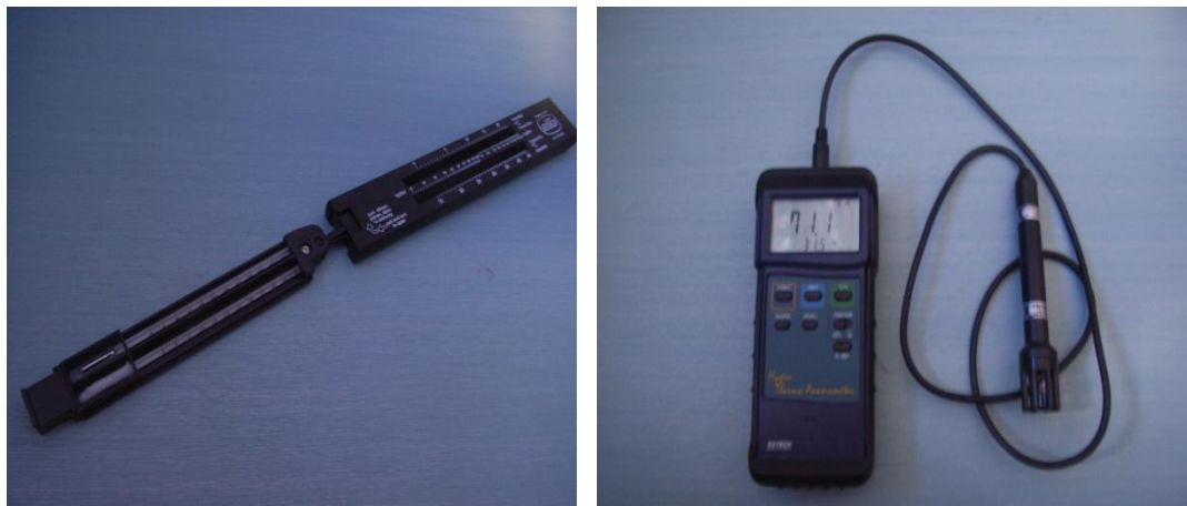
Figure 20: The humidity measuring device; hygrometer and anemometer.
