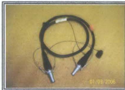
Figure 32: Short 5700 to TSCe Cable is use to connect receiver to TSCe.
