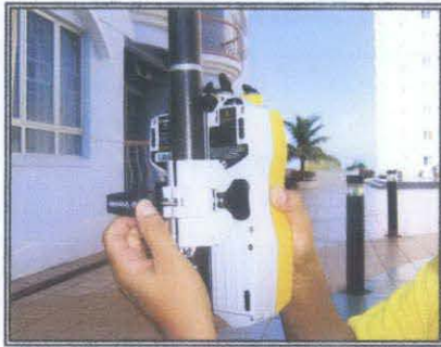
Figure 41: 5700 GPS receiver is attached to the lower part of the pole, and then locked the bracket to the pole.
