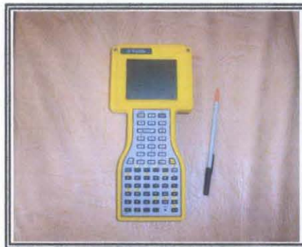
Figure 21: Trimble Survey Controller – TSCe and Pen Stylus. Data Logger has to equip with Window CE. The data will be display on TSCe screen.
