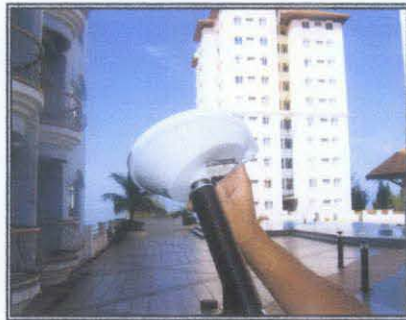
Figure 38: "Zephyr" antenna is set to the pole and make sure it is tighten
