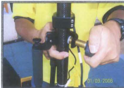
Figure 48: Setting the pole at station
