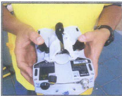
Figure 36: Pole mount bracket is attached at the back of 5700 GPS receiver
