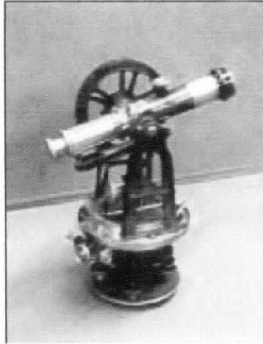
Figure 2: Telescopic level used in the early days of surveying ( http://www.surveyhistory.org/index.htm )
