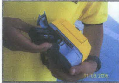
Figure 34: Battery is inserted to the receiver
