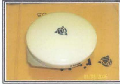
Figure 17: TRIMBLE rover antenna using dual-frequency without geodetic ground plane
