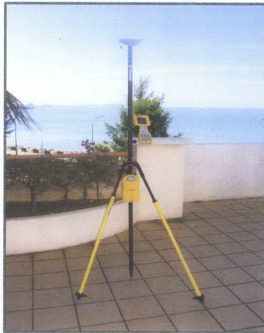
Figure 50: GPS RTK equipment that have been set up
