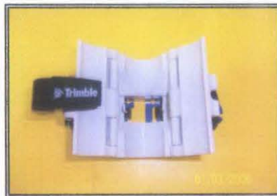
Figure 19: 5700 GPS Receiver Pole Mount Bracket were clipped to the Receiver. It is use to hold the Receiver to Range Pole
