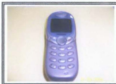
Figure 25: Hand phone. The purpose is to receive the corrected data from control centre at Geodesy section. The hand phone will be connected to TSCe during the surveying.
