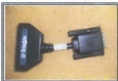
Figure 29: Multi port Adapter use to download data from TSCe to computer.
