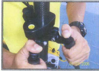
Figure 49: Adjusting the bubble to level the equipment
