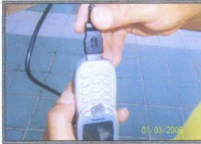
Figure 46: Cable RS232 is connected to hand phone
