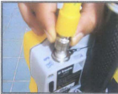
Figure 44: Cable antenna is connected to GPS Receiver port that indicate satellite symbol
