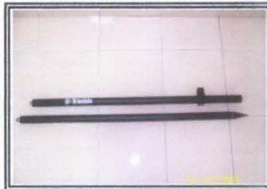
Figure 18: 2m height Carbon Fibre Range pole used to set up the rover unit during surveying. The spirit bubble at the middle of the pole is use to adjust the antenna placing.
