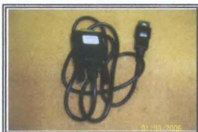
Figure 30: Cable RS232 used to connect hand phone to TSCe.
