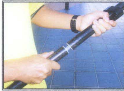
Figure 37: Both poles are joint and make sure the sharp ends were downward
