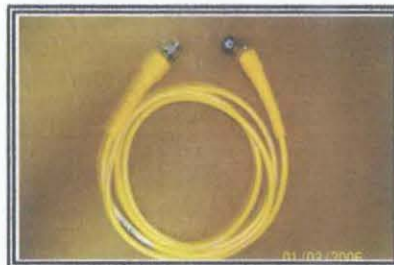
Figure 33: Antenna Cable use to connect receiver to antenna.
