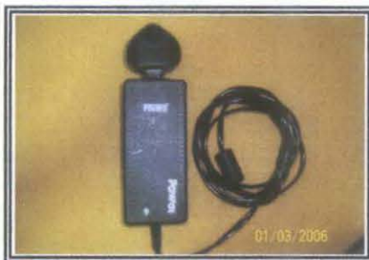
Figure 27: Power Supply Cable is used with Y-Cable to charge the Receiver battery and TSCe. It comes together with the GPS RTK set.
