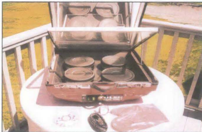
Figure 2.2 Tulsi-Hybrid Solar Oven Cooking Panel
