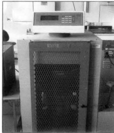
Figure 3.4: Compressive strength machine
