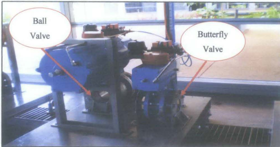
Figure 14: Ball Valve and Butterfly Valve
