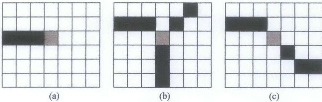
Figure 8: Minutiae Extraction (a) Termination (b) Bifurcation (c) Usual Pixel
