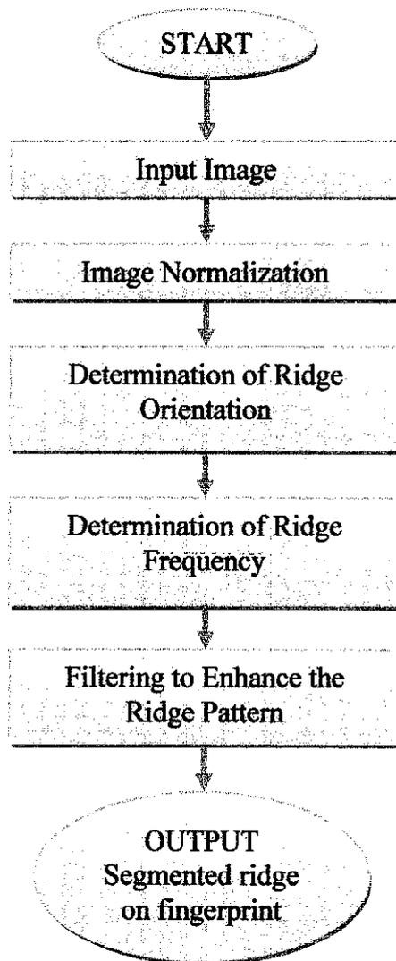
Figure 4: Enhancement Process Using Ridge Filter
