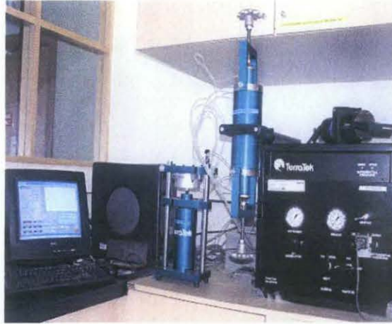
Figure 1. TerraTek PoroPerm to measure porosity and permeability.
