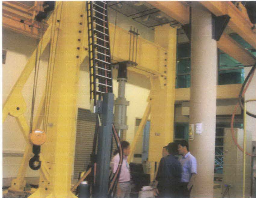
FIGURE 13: Compression test using UTM machine
