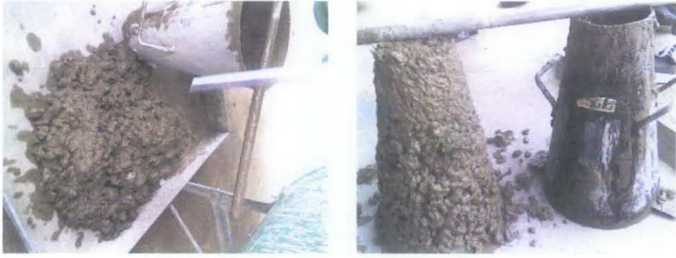
FIGURE 11: Slump test done on 0% PVA FRC (left) and 3% PVA FRC (right)
