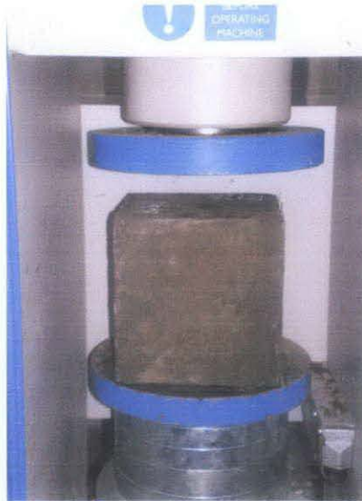
FIGURE 12: Compression test using compression machine
