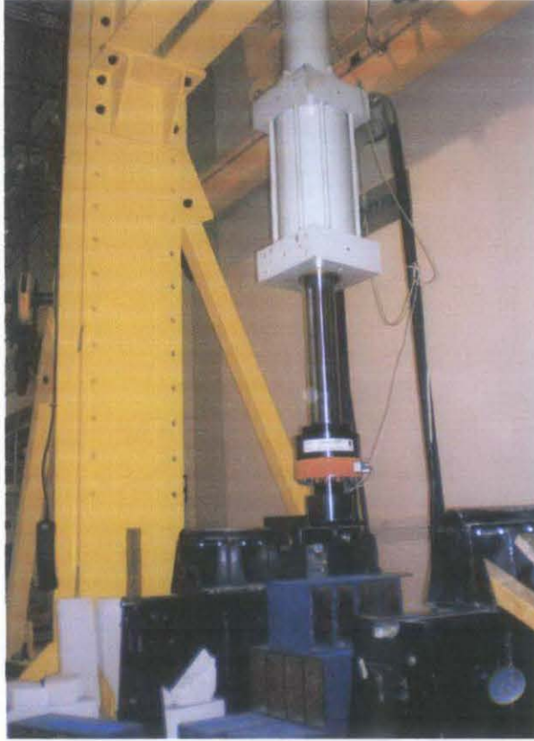
FIGURE 14: Compression test using UTM machine
