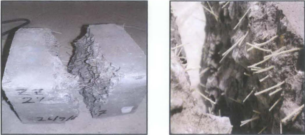
Figure 4.2.2d: Concrete cubes after the tests
