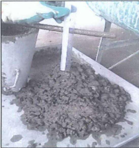
Slump test of PVA 0% concrete
