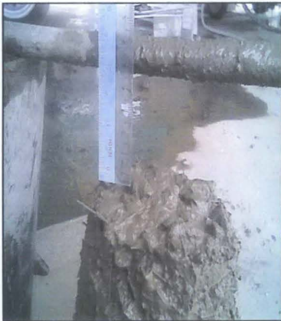
Slump test of PVA 2% concrete
