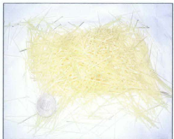
Figure 2.1c: Polyvinyl alcohol (PVA) fiber (RF 4000).
