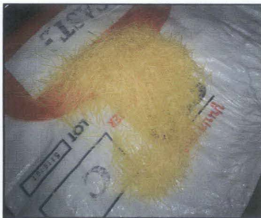
Figure 2.1c: Polyvinyl alcohol (PVA) fiber (RF 4000).
