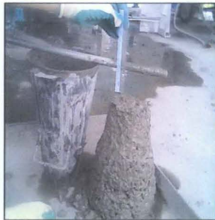
Figure 4.1.1b: Slump test of concrete with 1% PVA fiber
