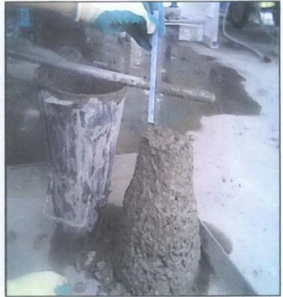
Slump test of PVA 1% concrete
