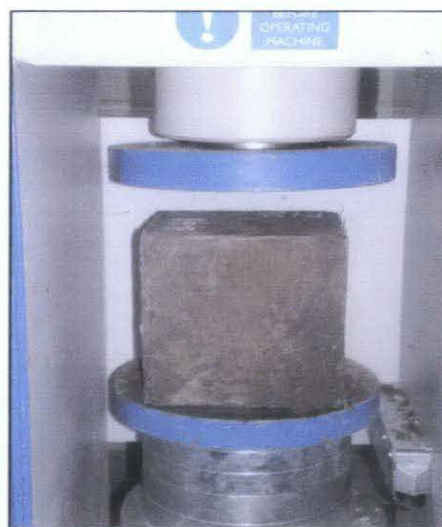
Figure 3.2.3b: Compressive Strength Test.
