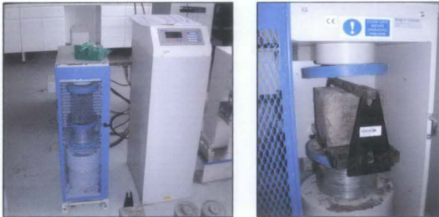
Figure 4.2.2a: Compression machine added with splitting tensile mould
