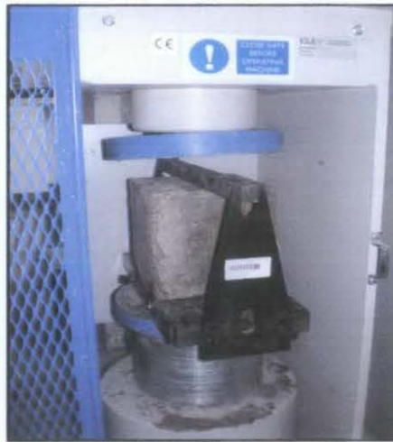
Figure 3.2.3c: Tensile Strength Test.
