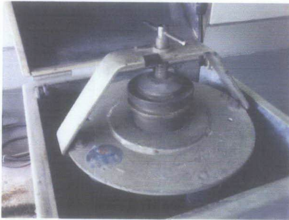
Figure A-3: Inside View of Rock Lab Granulator
