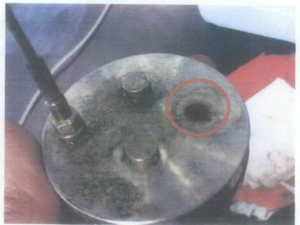
Figure A-6: Failure Part That Cause Explosion
