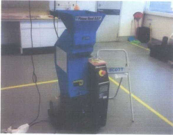
Figure A-1 Granulator
