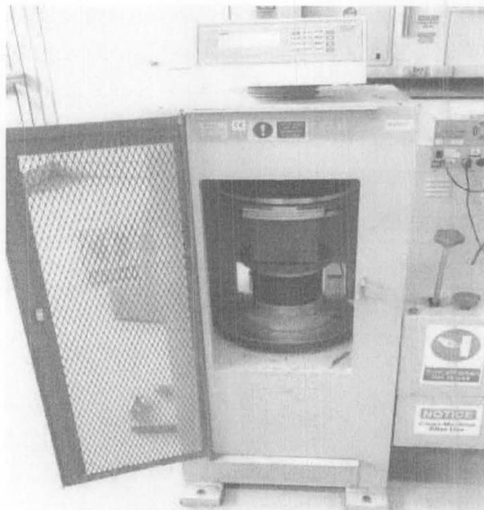
Fig. 3.5 CONCRETE CUBES UNDER TESTING
