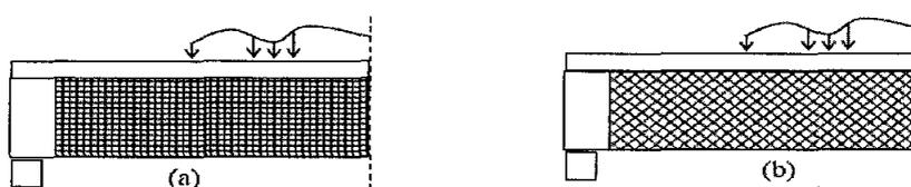
Fig. 2.9 BI-AXIAL FRP ORIENTATION. (a)  $90^{\circ}/0^{\circ}$ . (b)  $\pm 45^{\circ}$
