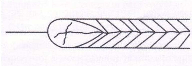
Figure 2.1: A schematic diagram of a centerline crack
