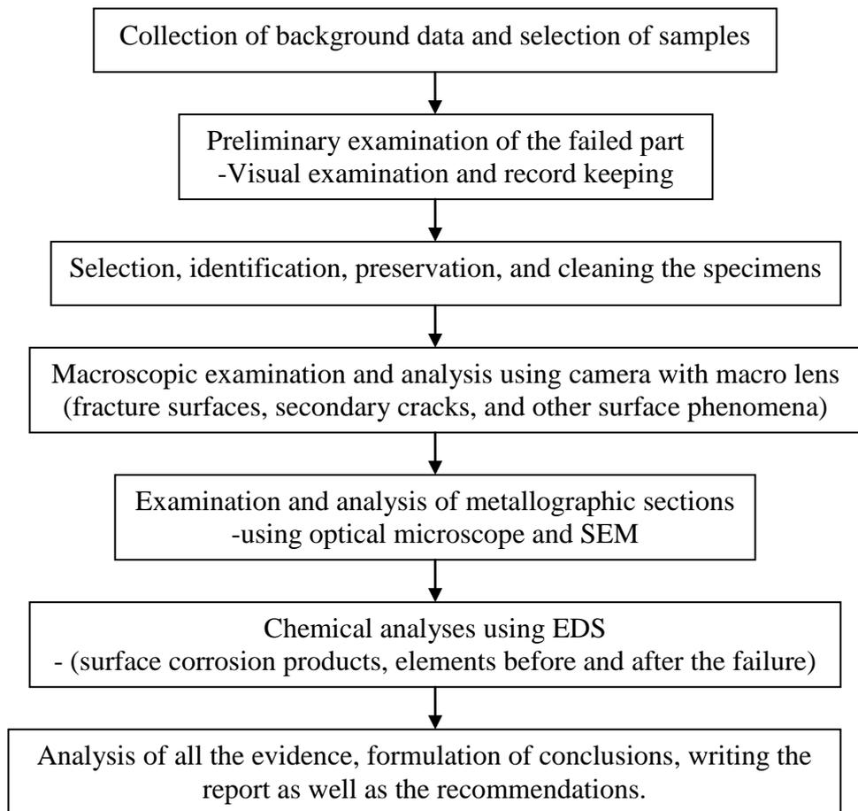
Figure 3.1. The flow of proper step to conduct failure analysis for this investigation
