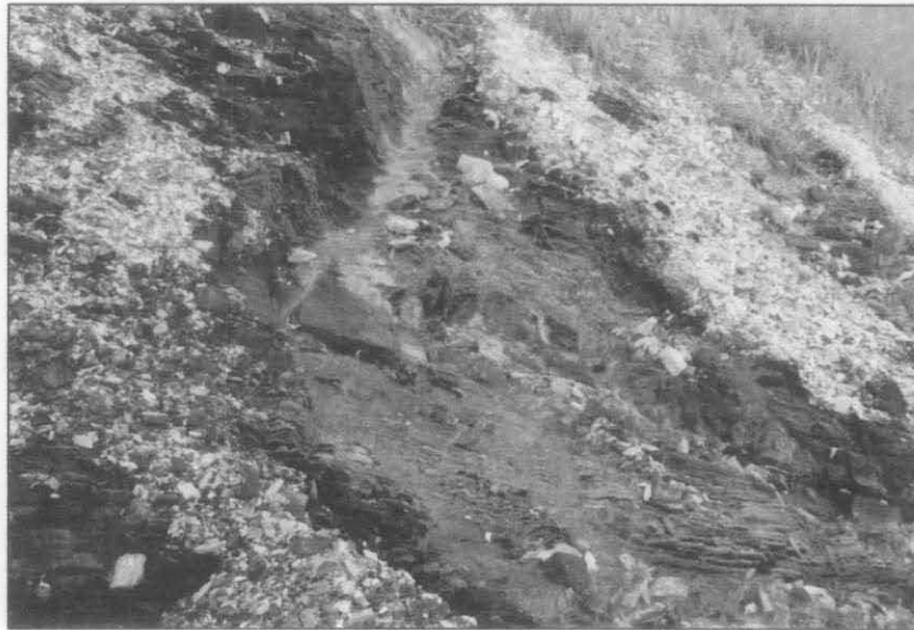
Figure 1: The effect of ARD on the carbonaceous shale
