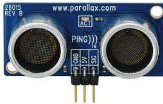
Figure 07: Ping - Ultrasonic Distance Sensor
