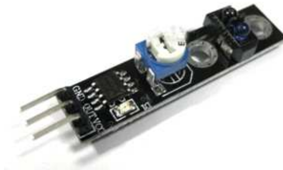
Figure 08: IR Line Tracking Sensor (Single Bit)
