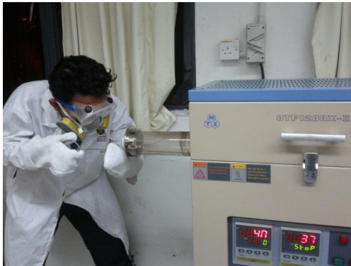
Pulling out the alumina boat after the nitriding process is done
