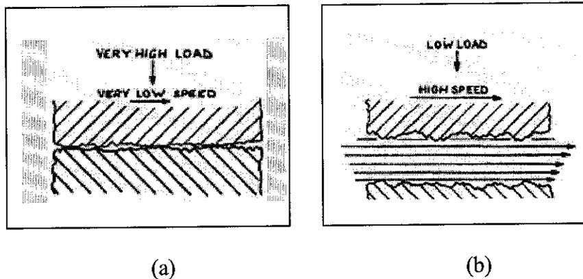
Figure 2.1 Lubrication system (a) Boundary Lubrication (b) Hydrodynamic Lubrication
