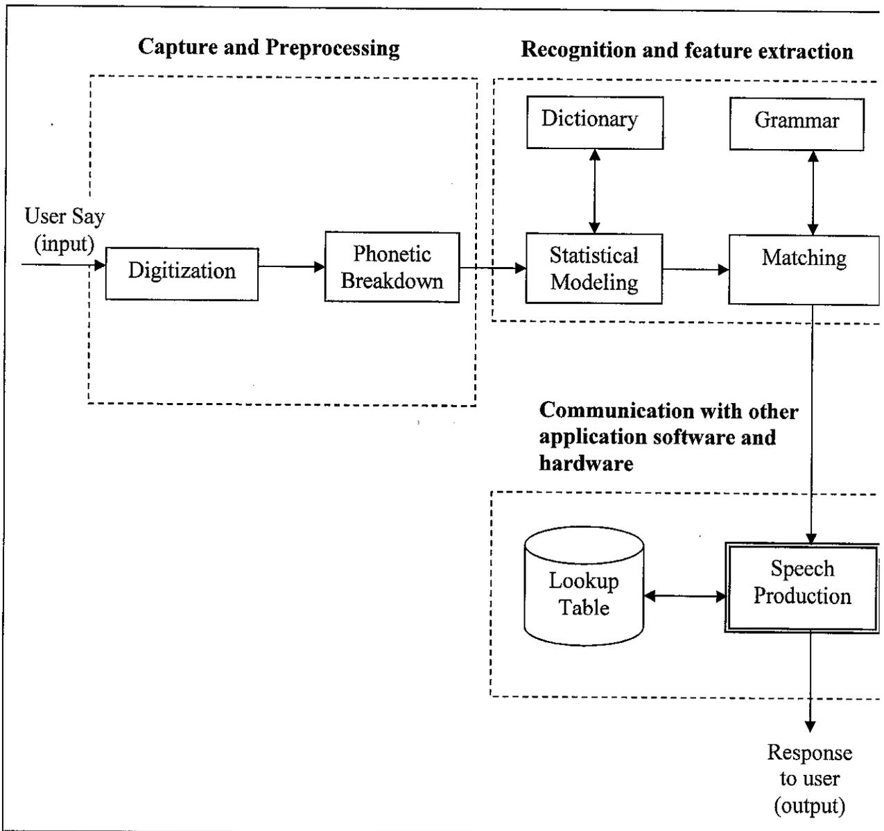
Figure 3.4 Combinations of Speech Component and VBBS Approach Flow
