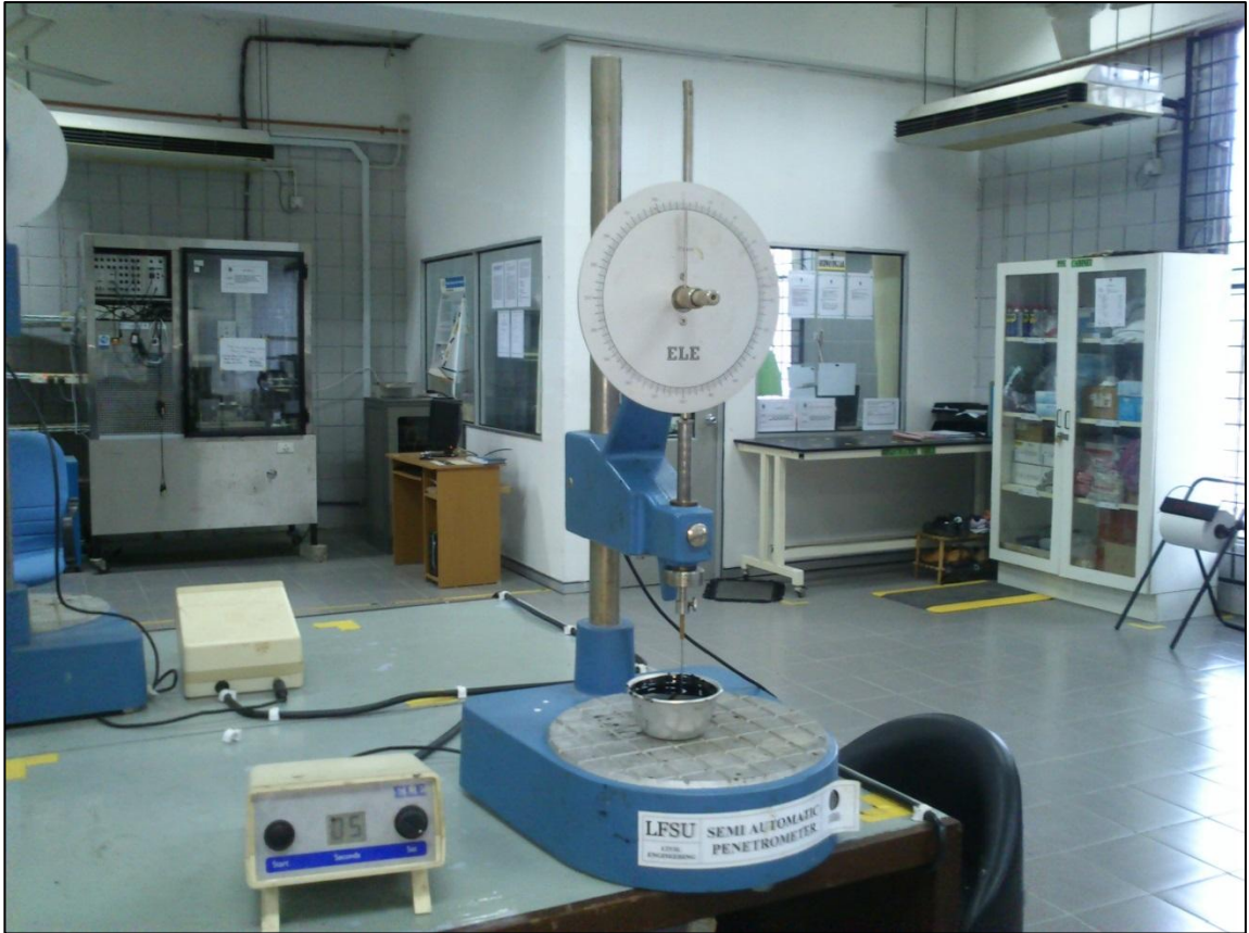
Figure 14: Penetration Test of the sample
