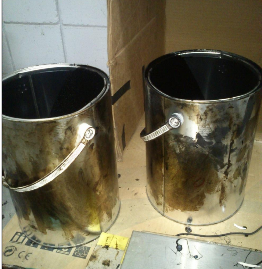
Figure 13: Cans used to Mix the Bitumen with Carbon Blacks
