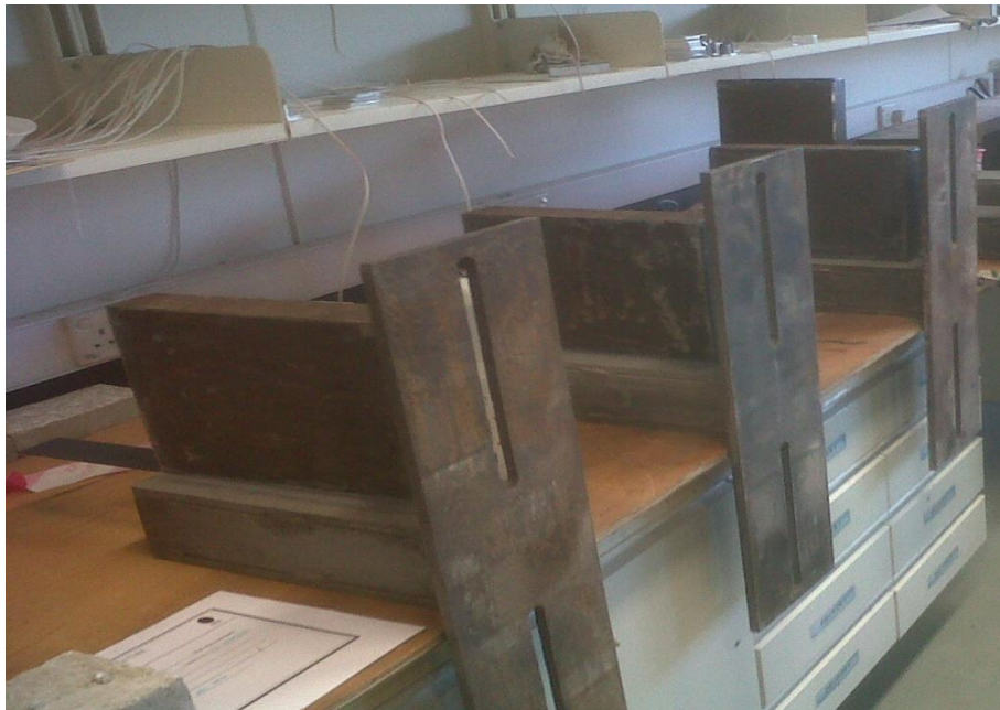
Figure 11. Curing process with 25kg steel block on the CFRP plate.
