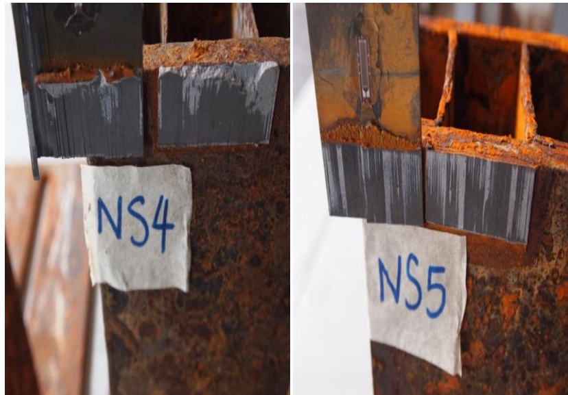
Figure 36: Failure mode of 1 month accelerated sea water for not fully anchored specimen
