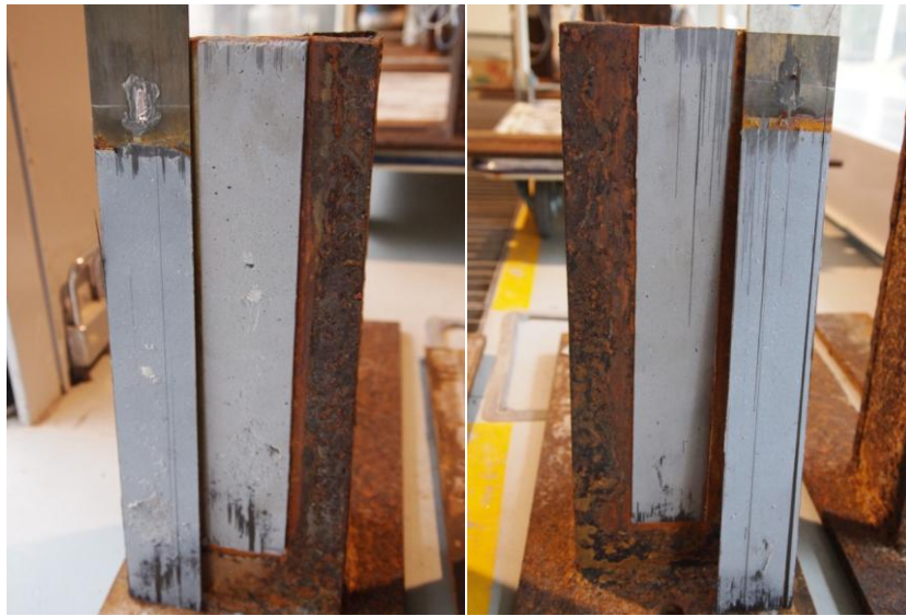
Figure 35: Failure mode of 1 month accelerated sea water for fully anchored specimen
