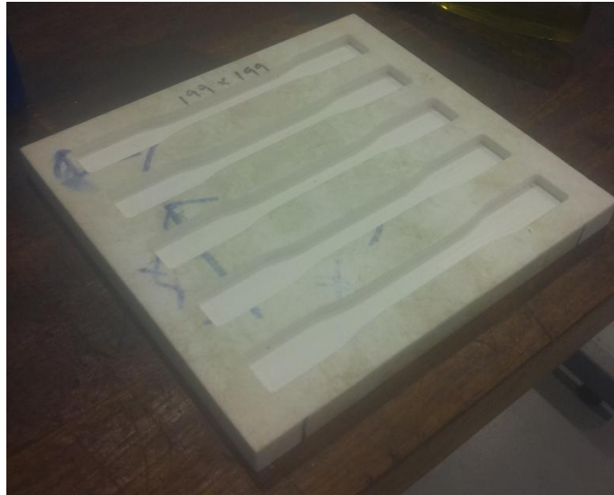
Figure 18: Mould for adhesive specimen's preparation
