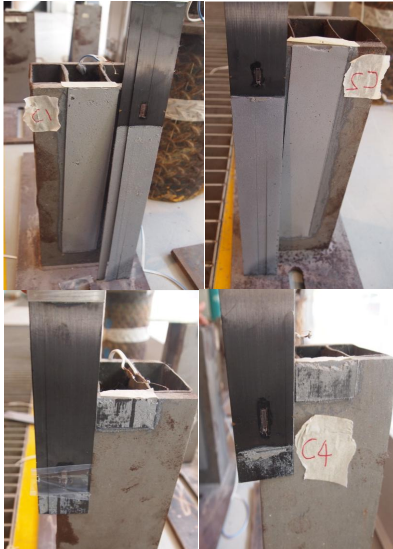
Figure 32: The failure modes of controlled specimens (fully anchored and not fully anchored)
