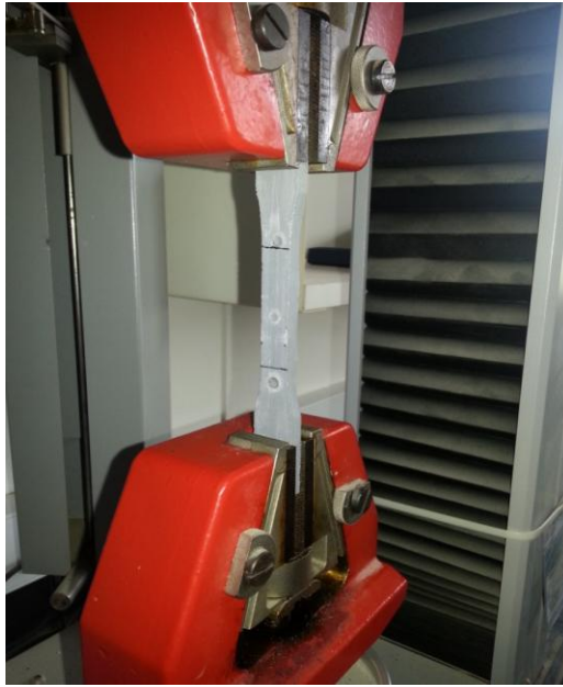
Figure 20: Test setups and instrumentation of dog-bone epoxy samples
