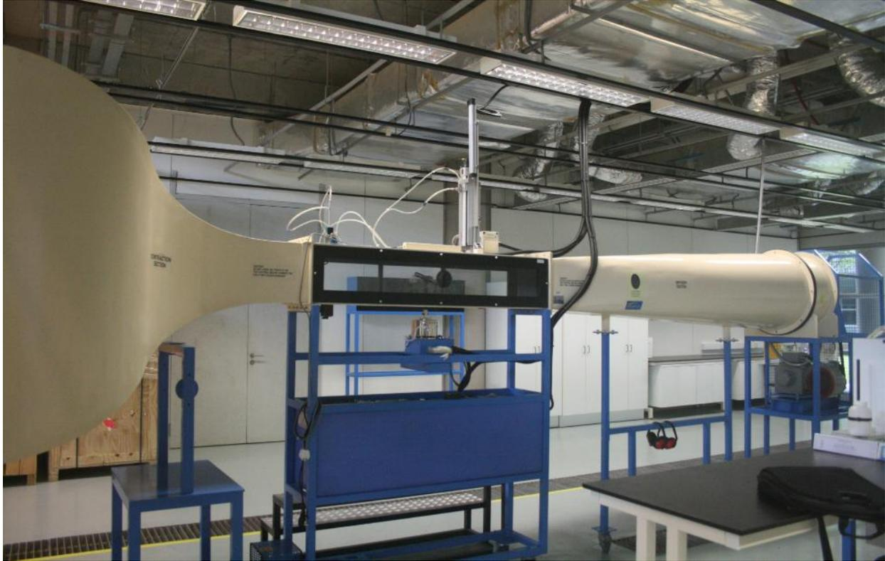
**Figure 4.1:** UTP open-circuit wind tunnel
