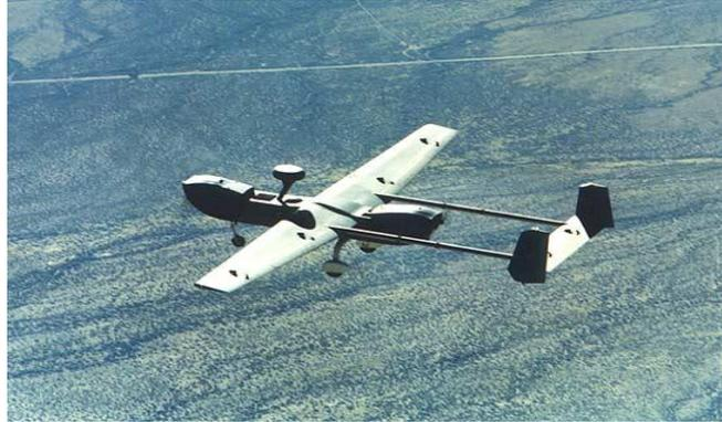
**FIGURE 1.3:** Example of medium size UAV-hunter 1 [6]
