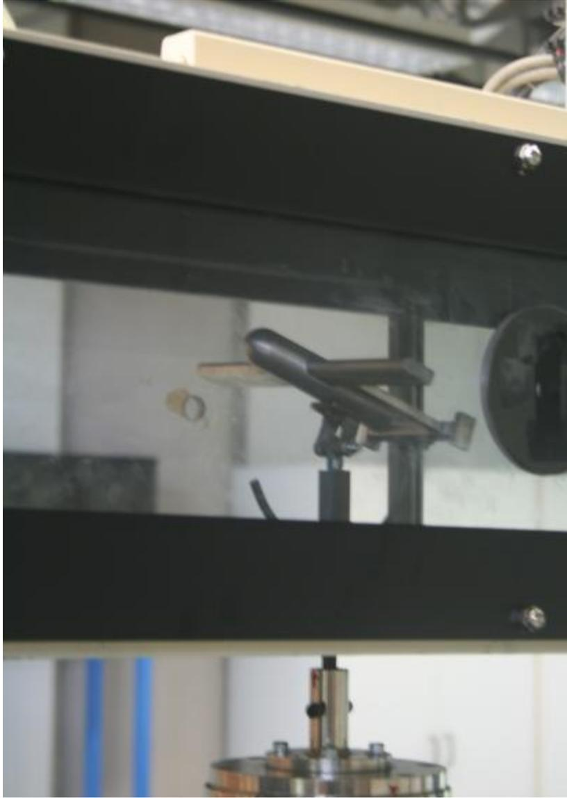
**Figure 4.8:** MAV in the wind tunnel testing section
