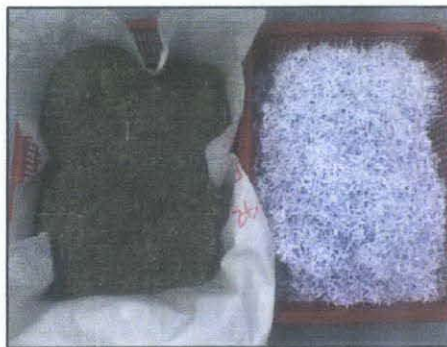
Figure 3.2: Grinded yard waste and shredded paper
