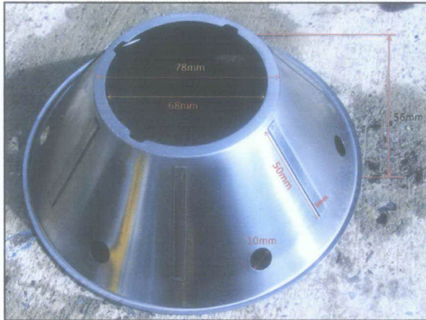
Figure 3.3: Top view of one of the cone in the centrifugal separator
