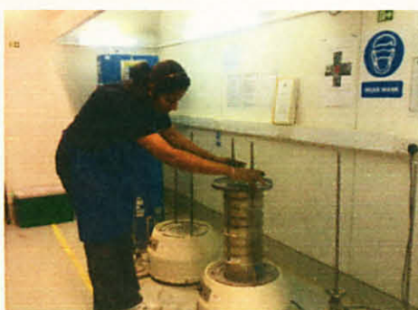
Figure 3.5: Conducting Sieve Analysis
