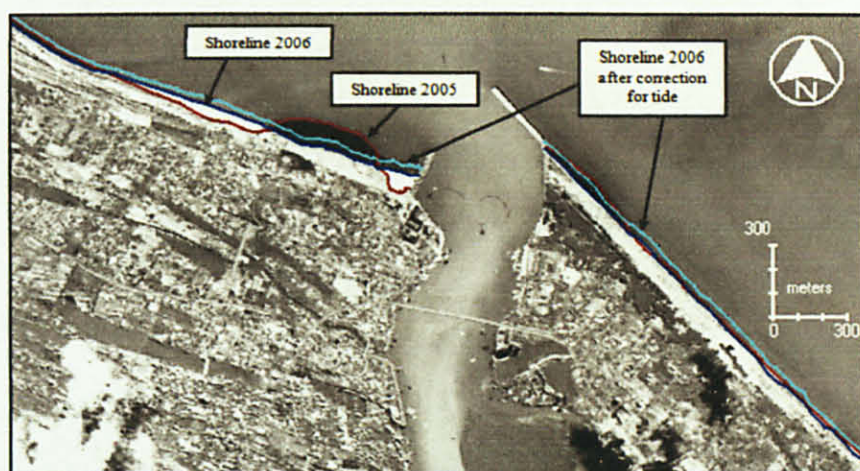
Figure 4.4: Shoreline change from 2005 to 2006 (tide corrected)
