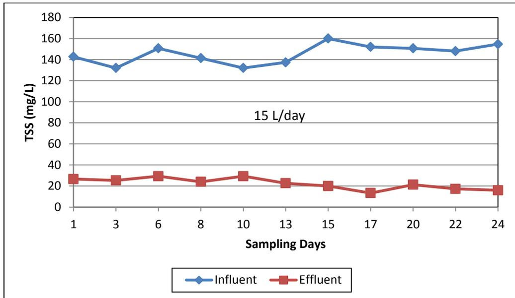
**Figure 25:** Graph of Total Suspended Solid (mg/L) vs Sampling Days
