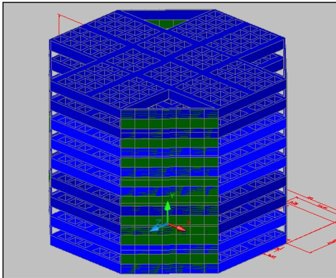
**Figure 8:** Final Design of the Aero-Packer Packing Medium
