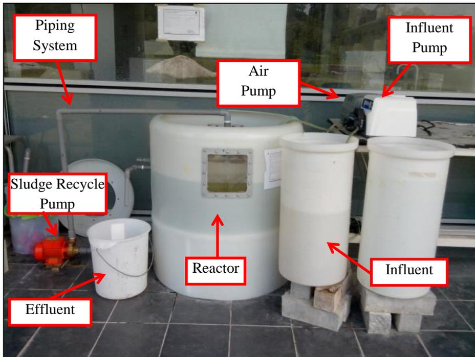
**Figure 6:** Setup Arrangement of the Reactor
