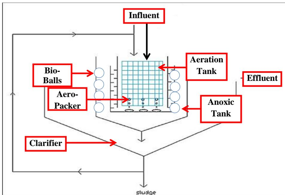
**Figure 9:** Schematic Diagram of the Reactor with Aero-Packer
