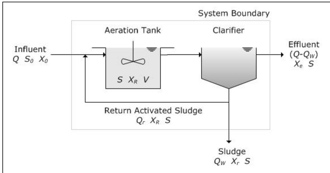
**Figure 1:** Activated Sludge Process Schematic Diagram (Lenntech B.V, 2008)
