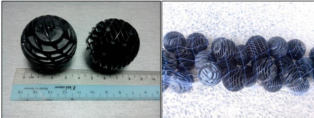
**Figure 14:** Configuration of the Bio-Balls
